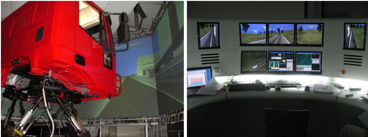
(a) Motorised simulator cabin, and projections panels
