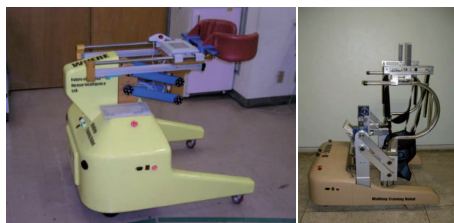
Figura 1.38: Los dispositivos WHERE I y II desarrollados en el Department of Electrical Engineering and Computer Science, Korea Advanced Institute of Science and Technology .
