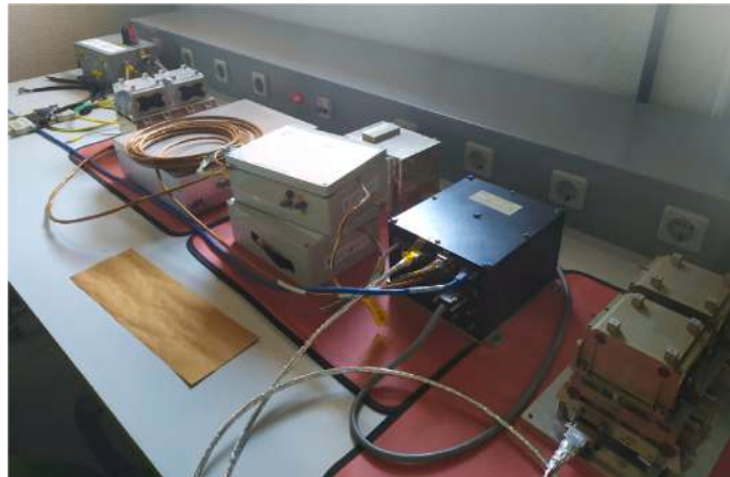
(c) EPD EQM ICU Test Scenario with 4 EQM sensors
