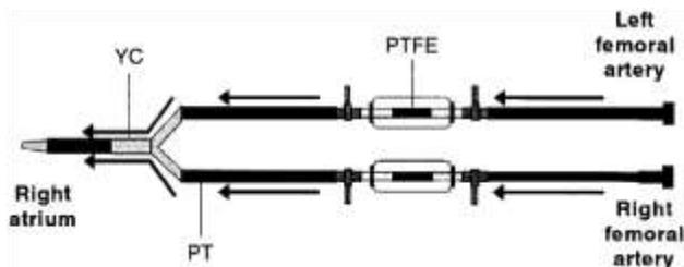
**Figure 1.** Femoro-atrial “*ex vivo*” circuit. PT: polyethylene tube; PTFE: polytetrafluoroethylene prostheses; YC: Yconnection; arrows indicate direction of blood flow.
