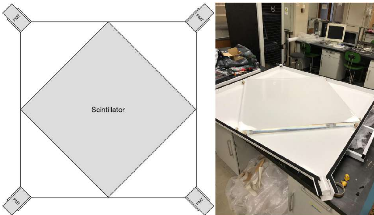
Fig. 1. On the left, scintillator, PMTs and pyramidal light guides configuration in each MITO device. On the right, scintillator inside the enclosure, which also serves as a light guide.
