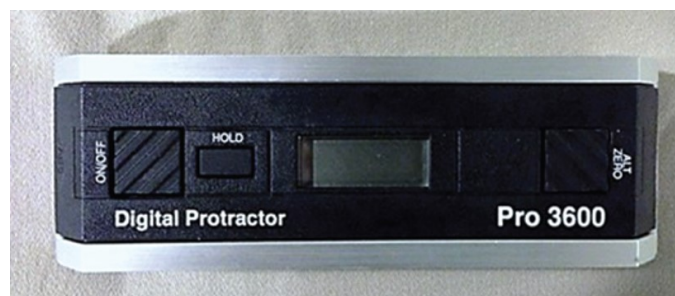
Fig. 2.45: Inclinómetro digital (Digital Protractor Pro 3600, Mitotoyo America, Aurora, IL, USA) Tomado de Roach S, San Juan JG, Suprak DN, Lyda M. Concurrent validity of digital inclinometer and universal goniometer in assessing passive hip mobility in healthy subjects. Int J Sports Phys Ther. 2013;8(5):680-8.
