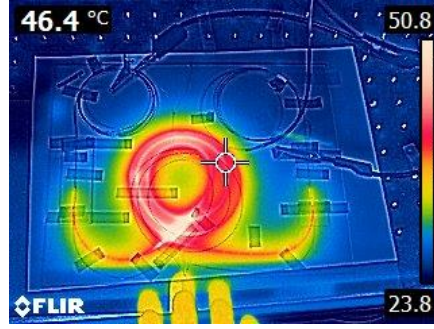
Fig. 1: Thermal infrared image of the sample optical fiber segment employed in the tests and the electrical contacts performed on the carbon coating to inject the electrical current. Around 3W/m were being dissipated when the image was taken.
