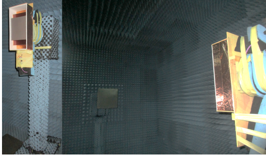
(a) Prototype assembled into anechoic chamber
