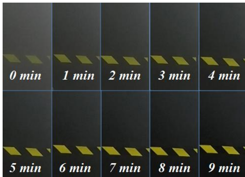
Time evolution of the fog generated with the F1:2 nozzle for a combination of P_{air}= 15 bar and P_{water}= 15 bar. The images show the concentration of fog in the room every minute since the shot was taken.
