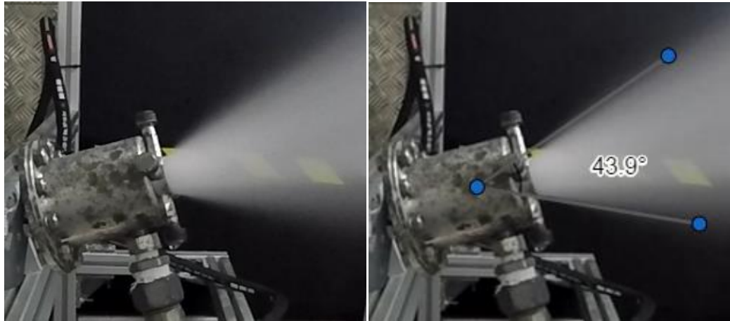
Stabilized cone of nozzle F1:2 for a P_{\text{air}}= 5 bar and P_{\text{water}}= 10 bar combination and cone opening angle.
