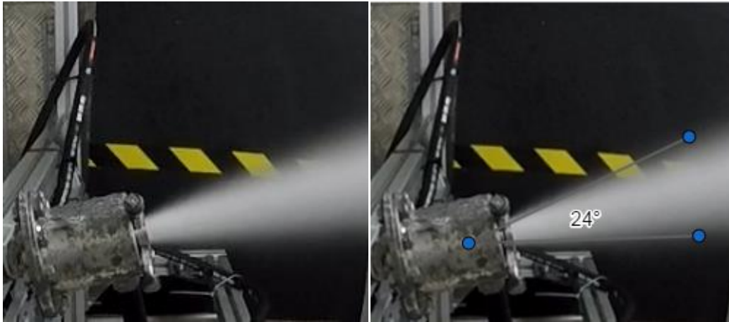
Stabilized cone of nozzle F1:2 for a P_{\text{air}}=20 bar and P_{\text{water}}=5 bar combination and cone opening angle.
