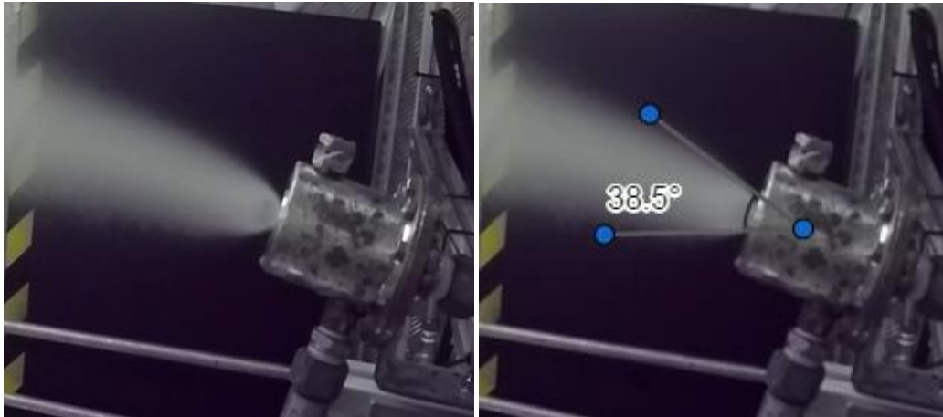
Stabilized cone of nozzle B1:2 for a P_{\text{air}}=7 bar and P_{\text{water}}=1.5 bar combination and cone opening angle.
