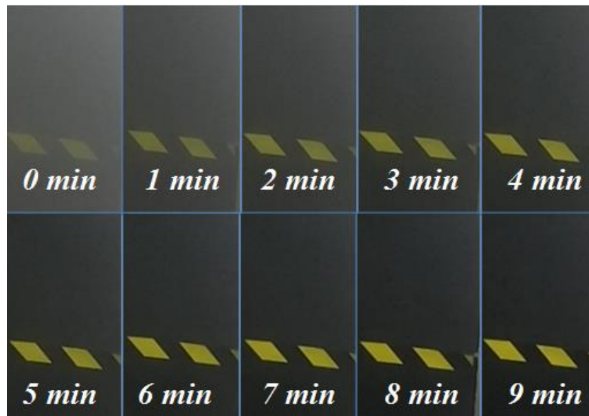
Time evolution of the fog generated with the F1:2 nozzle for a combination of P_{\text{air}}=5 bar and P_{\text{water}}=20 bar. The images show the concentration of fog in the room every minute since the shot was taken.
