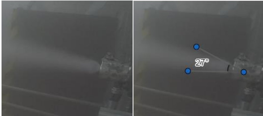
Stabilized cone of nozzle B1:2 for a P_{\text{air}}=19 bar and P_{\text{water}}=4 bar combination and cone opening angle.
