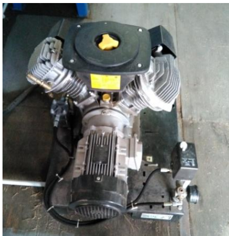
Figure 69: Pressurized air tank charge compressor
