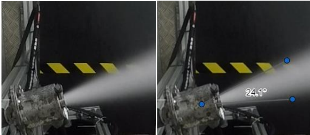
Stabilized cone of nozzle F1:2 for a P_{\text{air}}=15 bar and P_{\text{water}}=5 bar combination and cone opening angle.
