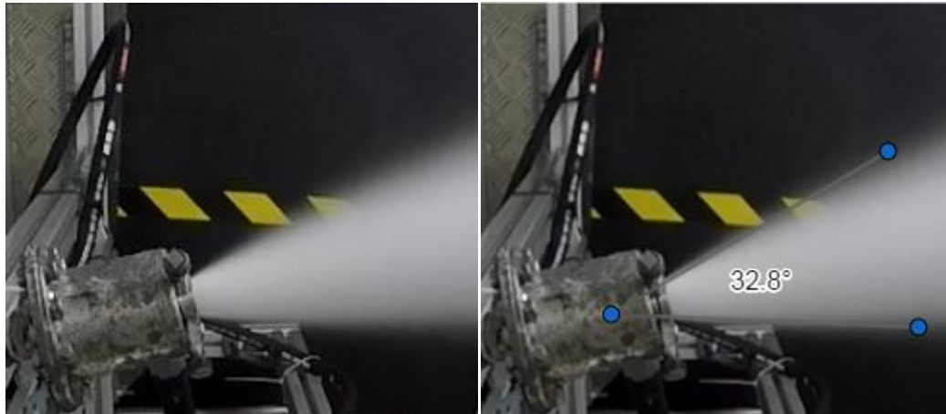
Stabilized cone of nozzle F1:2 for a P_{\text{air}}=20 bar and P_{\text{water}}=20 bar combination and cone opening angle.
