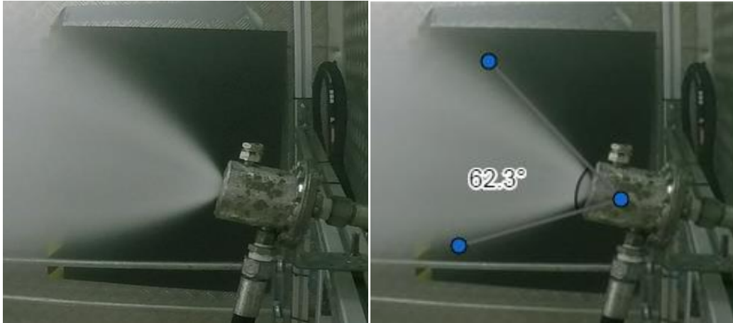
Stabilized cone of nozzle B1:2 for a P_{air}= 10 bar and P_{water}= 25 bar combination and cone opening angle.
