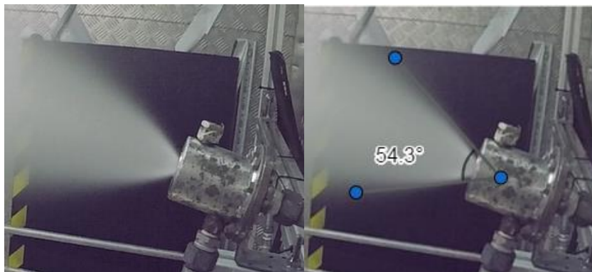
Figure 115: Stabilized cone of nozzle B1:2 for a P_{\text{air}} = 4.5 bar and P_{\text{water}} = 1.5 bar combination and cone opening angle.
