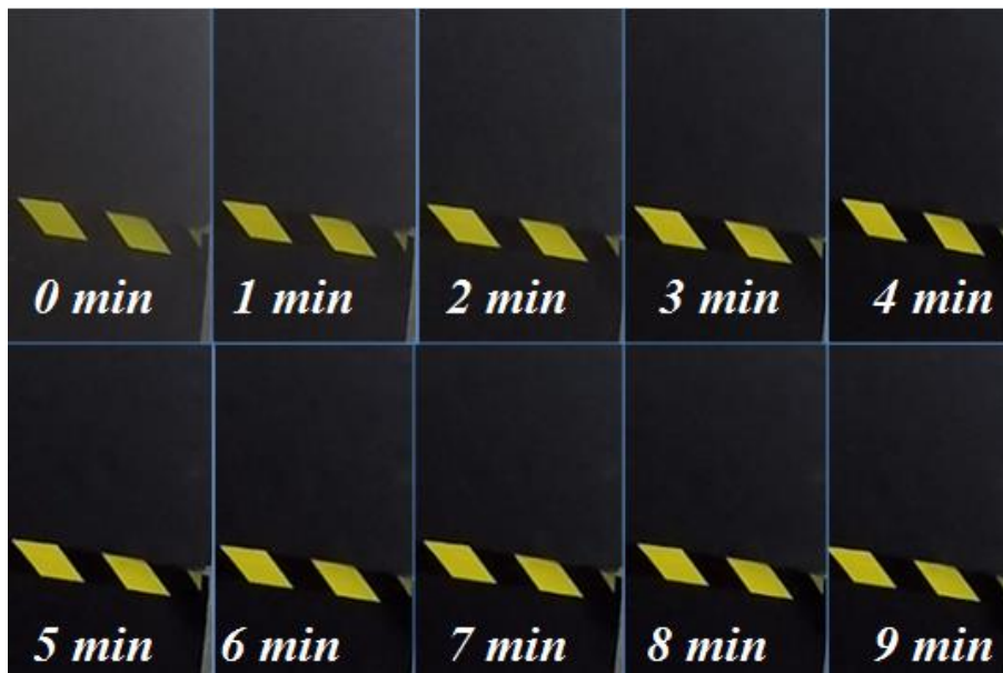
Time evolution of the fog generated with the F1:2 nozzle for a combination of P_{\text{air}}=10 bar and P_{\text{water}}=10 bar. The images show the concentration of fog in the room every minute since the shot was taken.
