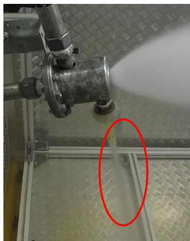
Figure 144: Some of the air and water flow generated inside the nozzle is expelled from the nozzle through the third component inlet.
