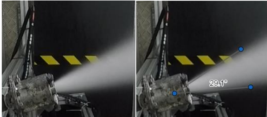
Stabilized cone of nozzle F1:2 for a P_{\text{air}}= 15 bar and P_{\text{water}}= 10 bar combination and cone opening angle.
