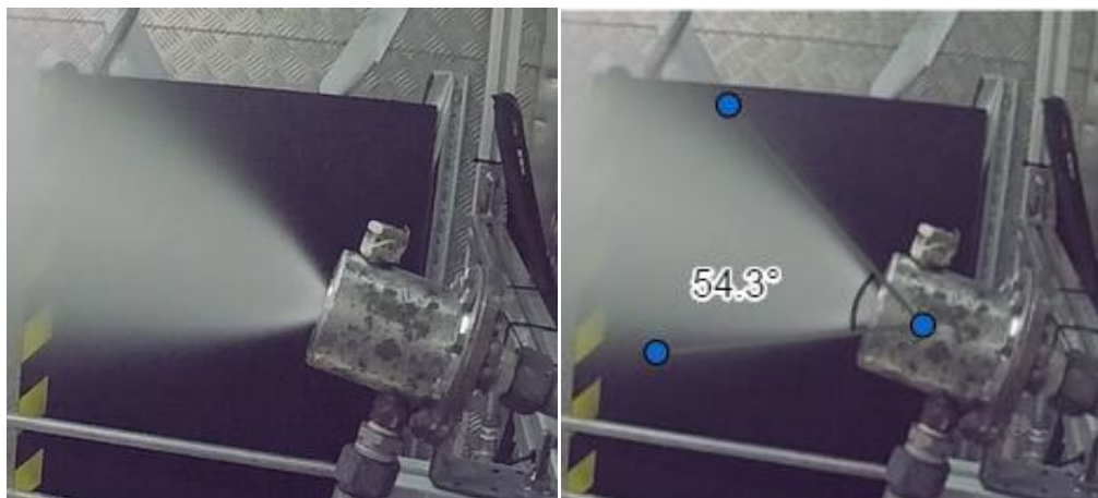
Stabilized cone of nozzle B1:2 for a P_{\text{air}}= 4.5 bar and P_{\text{water}}= 1.5 bar combination and cone opening angle.
