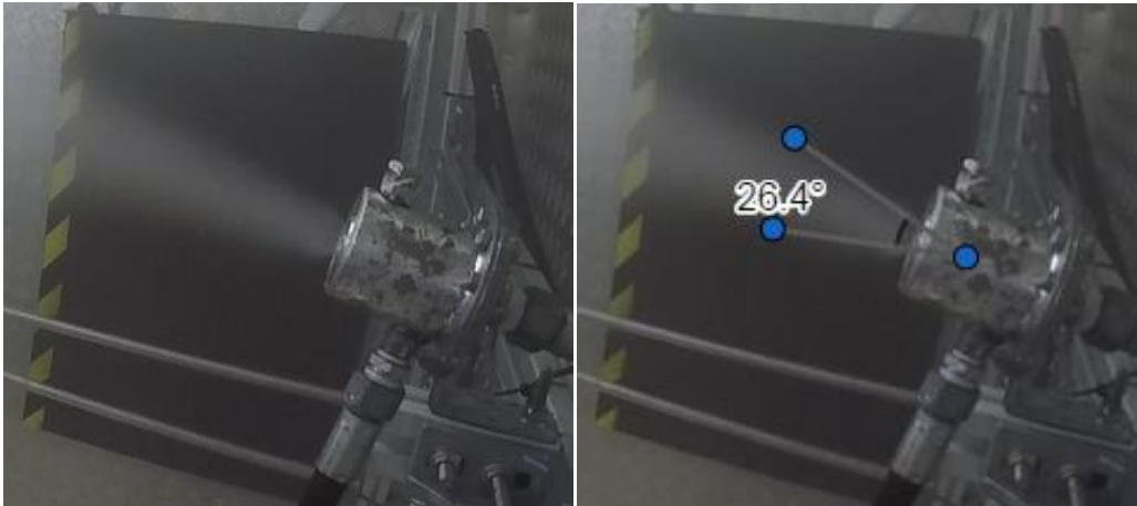
Stabilized cone of nozzle B1:2 for a P_{\text{air}}=9 bar and P_{\text{water}}=1.5 bar combination and cone opening angle.
