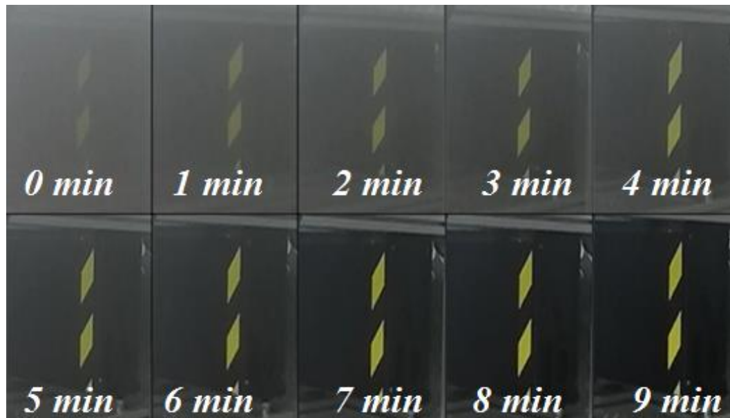
Time evolution of the fog generated with the B1:2 nozzle for a combination of P_{\text{air}} = 8 bar and P_{\text{water}} = 1.5 bar. The images show the concentration of fog in the room every minute since the shot was taken.
