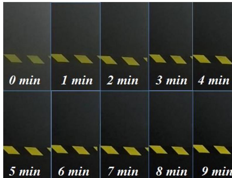
Time evolution of the fog generated with the F1:2 nozzle for a combination of P_{\text{air}}= 15 bar and P_{\text{water}}= 10 bar. The images show the concentration of fog in the room every minute since the shot was taken.
