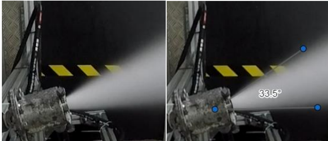
Stabilized cone of nozzle F1:2 for a P_{air}= 15 bar and P_{water}= 15 bar combination and cone opening angle.
