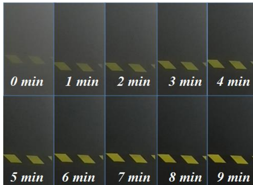
Time evolution of the fog generated with the F1:2 nozzle for a combination of P_{\text{air}}= 15 bar and P_{\text{water}}= 20 bar. The images show the concentration of fog in the room every minute since the shot was taken.
