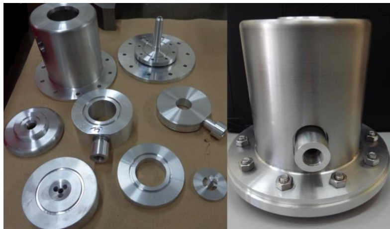
Figure 31: B1:1 nozzle parts and complete assembly
