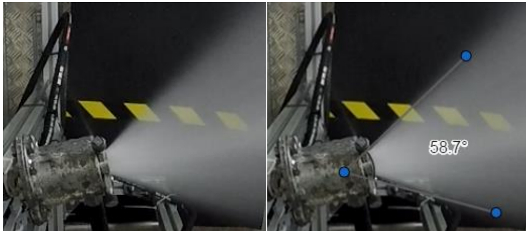
Stabilized cone of nozzle F1:2 for a P_{\text{air}}=5 bar and P_{\text{water}}=20 bar combination and cone opening angle.
