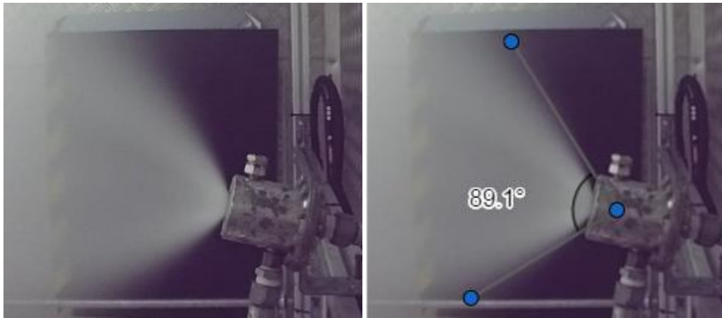
Stabilized cone of nozzle B1:2 for a P_{air}= 5 bar and P_{water}= 25 bar combination and cone opening angle.
