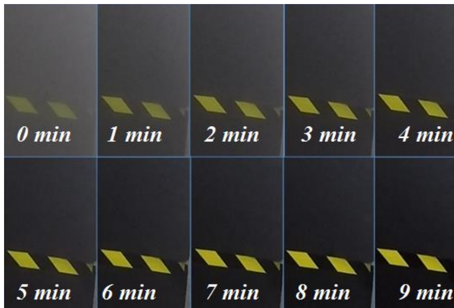
Time evolution of the fog generated with the F1:2 nozzle for a combination of P_{air}= 10 bar and P_{water}= 15 bar. The images show the concentration of fog in the room every minute since the shot was taken.
