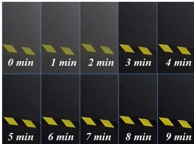
Time evolution of the fog generated with the F1:2 nozzle for a combination of P_{\text{air}}= 5 bar and P_{\text{water}}= 15 bar. The images show the concentration of fog in the room every minute since the shot was taken.
