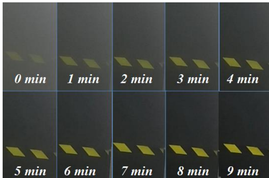
Time evolution of the fog generated with the F1:2 nozzle for a combination of P_{\text{air}}=20 bar and P_{\text{water}}=20 bar. The images show the concentration of fog in the room every minute since the shot was taken.
