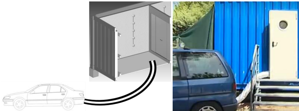
Figure 160: Introduction of the gases resulting from the combustion of the four-stroke Diesel engine.
