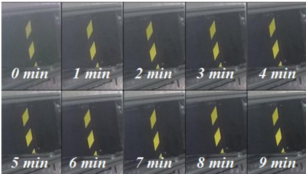
Time evolution of the fog generated with the B1:2 nozzle for a combination of P_{\text{air}}= 10 bar and P_{\text{water}}= 15 bar. The images show the concentration of fog in the room every minute since the shot was taken.
