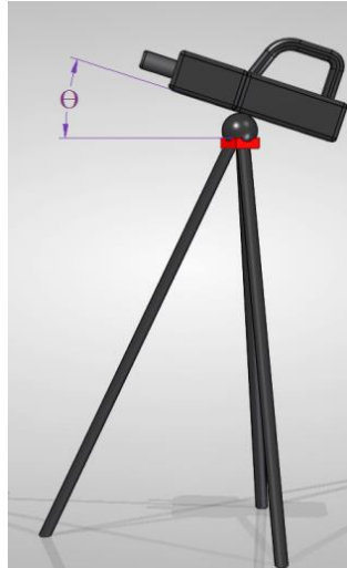
Figure 123: Pitch angle of the particle counter.
