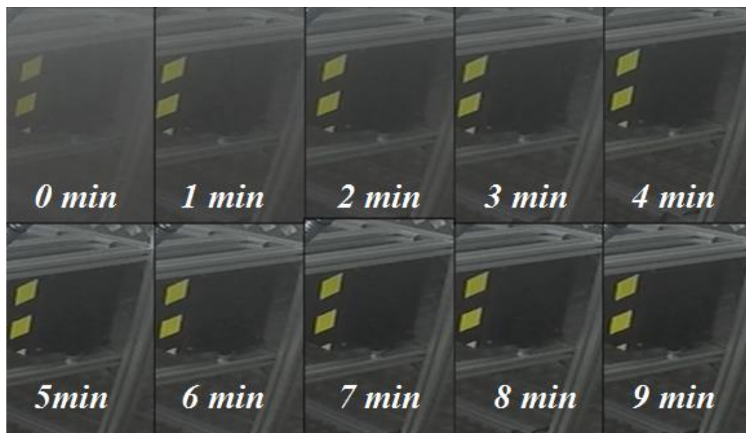
Time evolution of the fog generated with the B1:2 nozzle for a combination of P_{\text{air}}= 4.5 bar and P_{\text{water}}= 1.5 bar. The images show the concentration of fog in the room every minute since the shot was taken.
