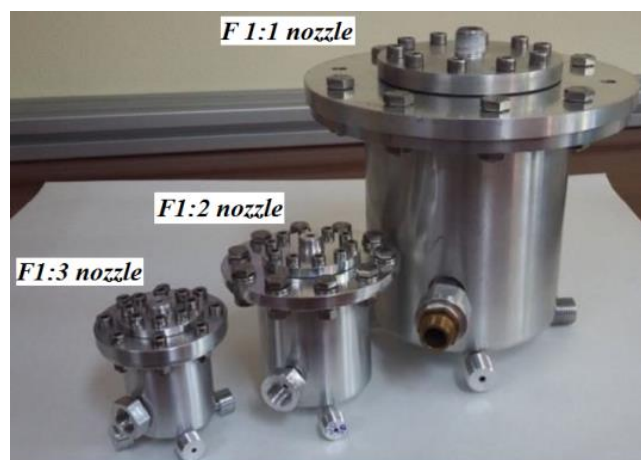
Figure 34: B nozzle model at different scales
