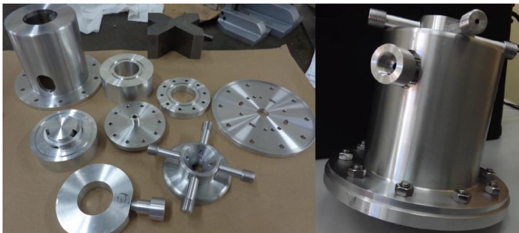
Figure 32: F1:1 nozzle parts and complete assembly
