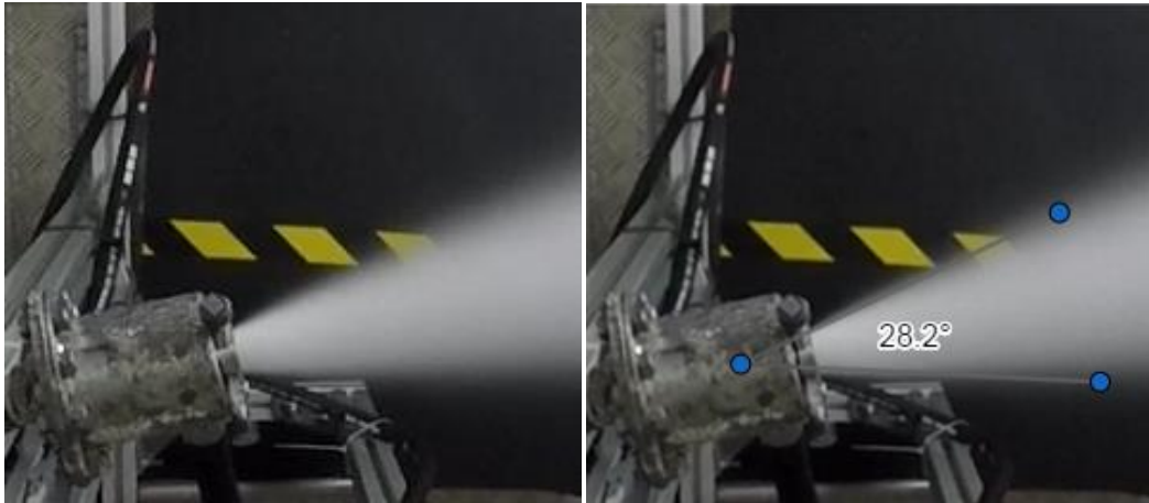
Stabilized cone of nozzle F1:2 for a P_{air}= 20 bar and P_{water}= 15 bar combination and cone opening angle.
