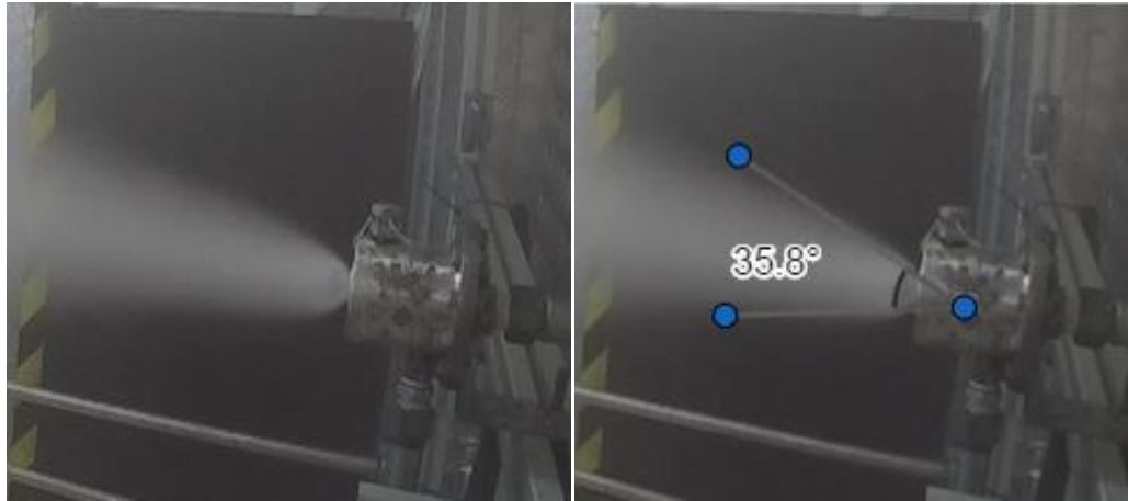
Stabilized cone of nozzle B1:2 for a P_{\text{air}}=12 bar and P_{\text{water}}=3 bar combination and cone opening angle.
