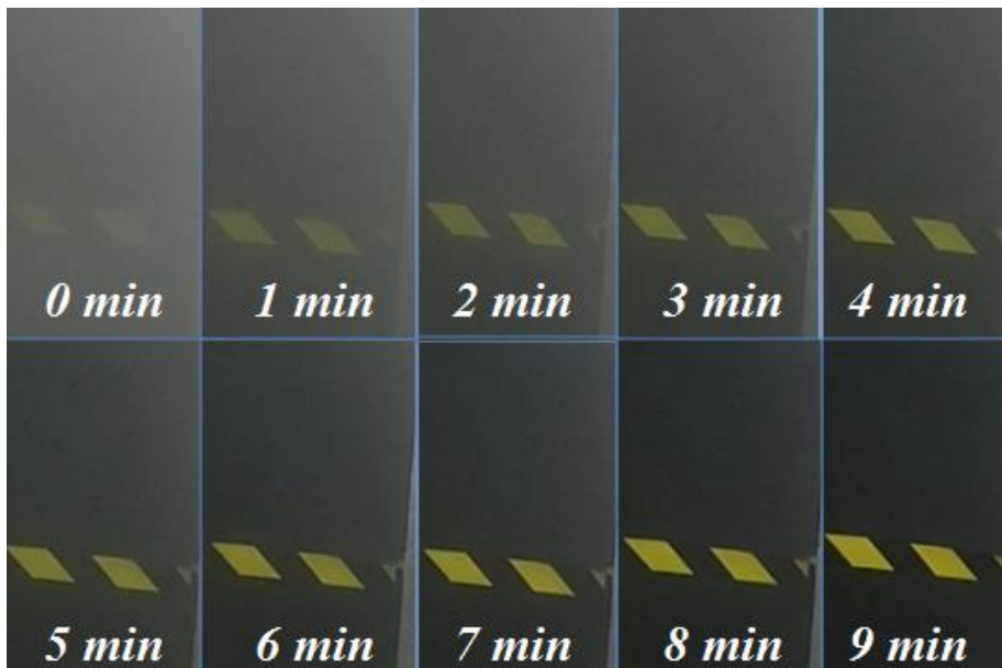
Time evolution of the fog generated with the F1:2 nozzle for a combination of P_{air}= 20 bar and P_{water}= 15 bar. The images show the concentration of fog in the room every minute since the shot was taken.
