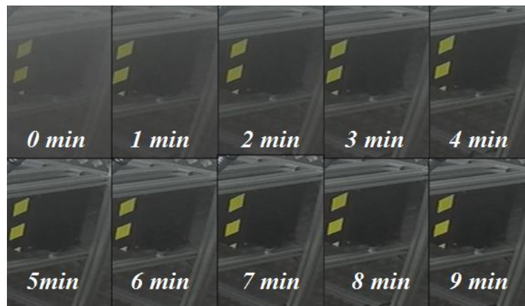
Figure 116: Time evolution of the fog generated with the B1:2 nozzle for a combination of P_{\text{air}} = 4.5 bar and P_{\text{water}} = 1.5 bar. The images show the concentration of fog in the room every minute since the shot was taken.
