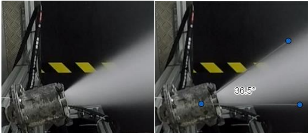
Stabilized cone of nozzle F1:2 for a P_{\text{air}}= 15 bar and P_{\text{water}}= 20 bar combination and cone opening angle.
