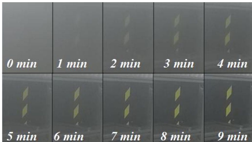
Time evolution of the fog generated with the B1:2 nozzle for a combination of P_{\text{air}}=19 bar and P_{\text{water}}=4 bar. The images show the concentration of fog in the room every minute since the shot was taken.
