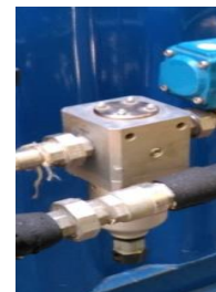
Figure 89: Manual air pressure regulation valve
