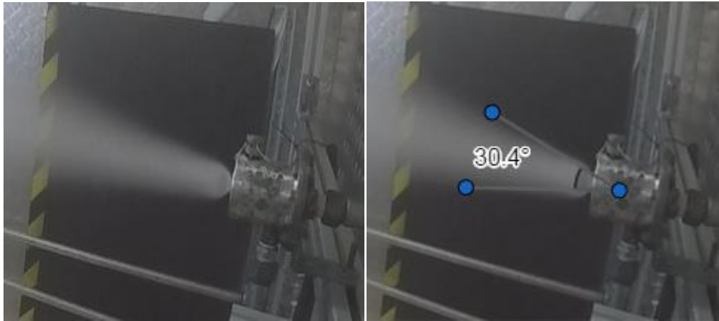
Stabilized cone of nozzle B1:2 for a P_{\text{air}}=15 bar and P_{\text{water}}=3 bar combination and cone opening angle.
