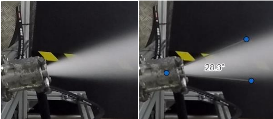
Stabilized cone of nozzle F1:2 for a P_{\text{air}}=10 bar and P_{\text{water}}=10 bar combination and cone opening angle.
