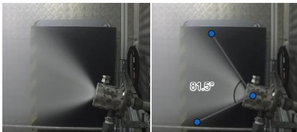
Stabilized cone of nozzle B1:2 for a P_{\text{air}} = 5 bar and P_{\text{water}} = 20 bar combination and cone opening angle.
