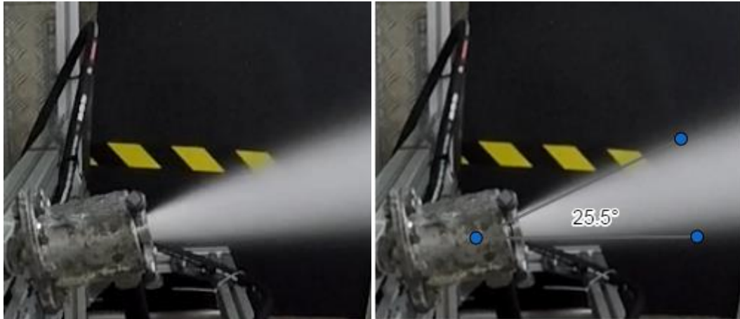
Stabilized cone of nozzle F1:2 for a P_{\text{air}}=20 bar and P_{\text{water}}=10 bar combination and cone opening angle.
