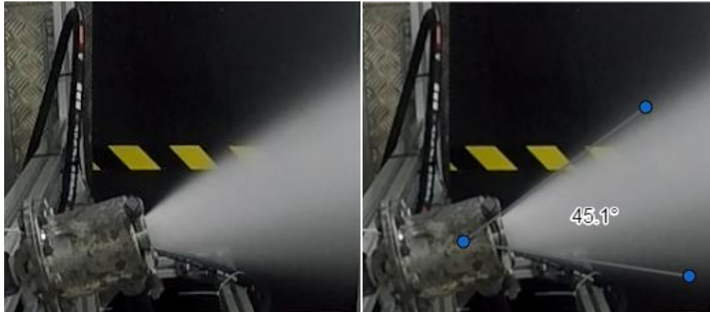
Stabilized cone of nozzle F1:2 for a P_{\text{air}}= 10 bar and P_{\text{water}}= 20 bar combination and cone opening angle.
