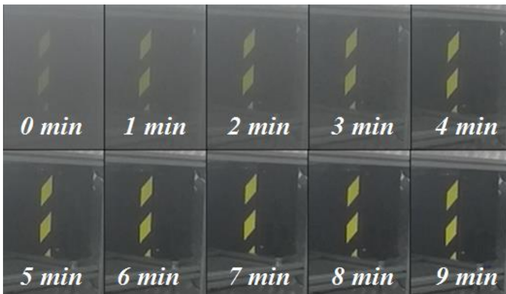
Time evolution of the fog generated with the B1:2 nozzle for a combination of P_{\text{air}}=9 bar and P_{\text{water}}=1.5 bar. The images show the concentration of fog in the room every minute since the shot was taken.
