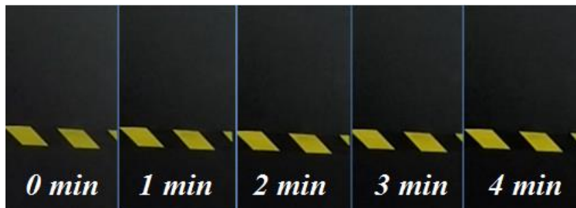
Time evolution of the fog generated with the F1:2 nozzle for a combination of P_{\text{air}}=15 bar and P_{\text{water}}=5 bar. The images show the concentration of fog in the room every minute since the shot was taken.
