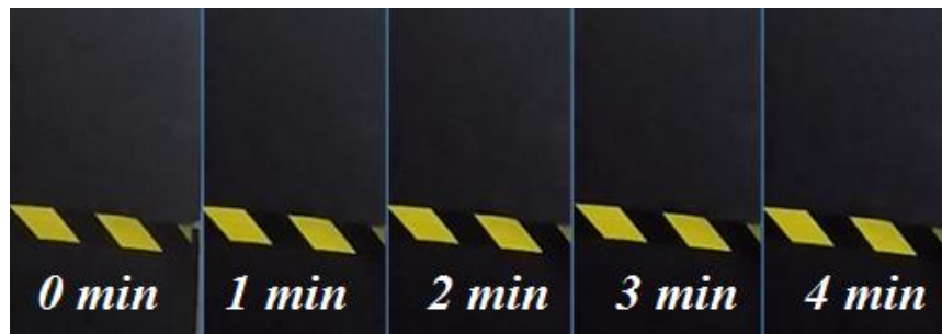
Time evolution of the fog generated with the F1:2 nozzle for a combination of P_{\text{air}}= 5 bar and P_{\text{water}}= 10 bar. The images show the concentration of fog in the room every minute since the shot was taken.
