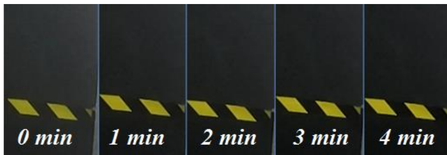
Time evolution of the fog generated with the F1:2 nozzle for a combination of P_{\text{air}}=20 bar and P_{\text{water}}=5 bar. The images show the concentration of fog in the room every minute since the shot was taken.
