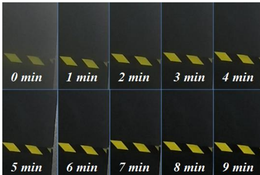
Time evolution of the fog generated with the F1:2 nozzle for a combination of P_{\text{air}}=20 bar and P_{\text{water}}=10 bar. The images show the concentration of fog in the room every minute since the shot was taken.
