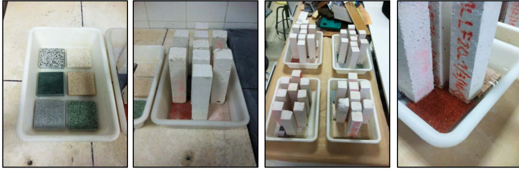
Fig. 1 Experimental setup for measuring capillary water absorption coefficients
