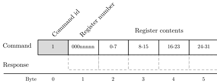
Figure 4.36: Register write command format.
