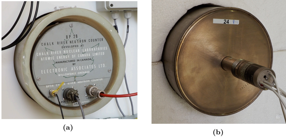
Figure 5.8: NEMO counter tube headers, BP28 (left) and LND2061 (right).
