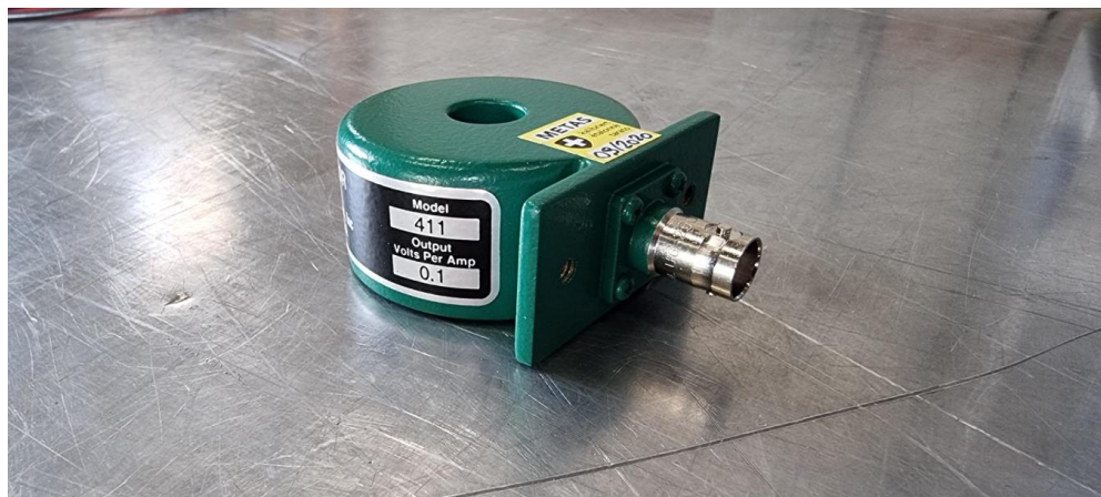
Figura 25: Vista general de la sonda PEARSON CURRENT MONITOR 411 .
