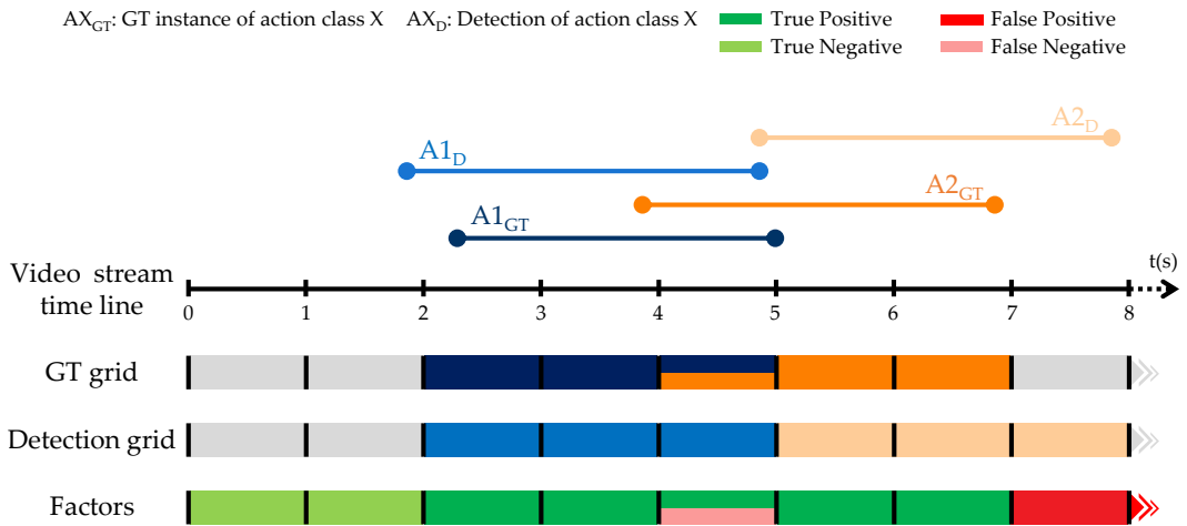
Figure 4.3: Instantaneous Accuracy implementation. Illustrative example of how the slot, the grid and the factors are actually built before computing the Instantaneous Accuracy during a certain part of a video. Here, the slot is configured to 1 second and the slot coverage threshold is 50%.
