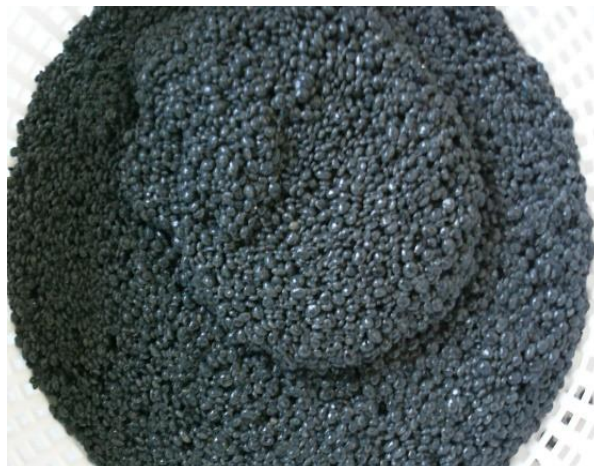
Fig.22 Lodo granular aerobio (AGS) ( www.globalwe.com )
