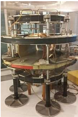
Figure 1. First MRI scanner build in 1980.
