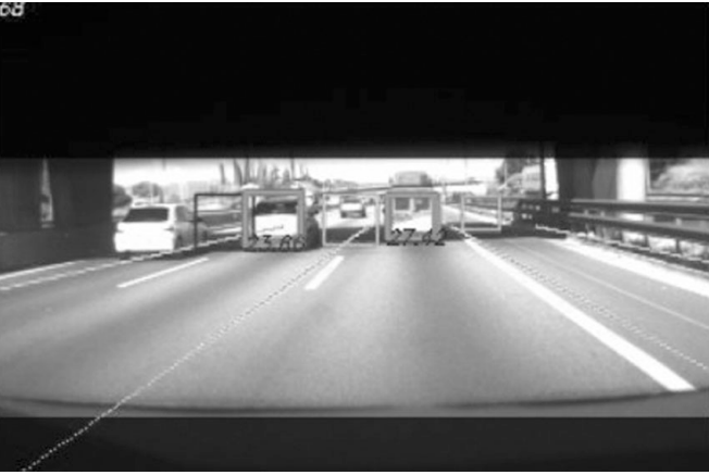
Fig. 22. Example of false vehicle detection.
