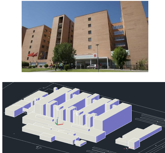
Figure 2. 3D image prior to the energy simulation of the Principe of Asturias Hospital of Alcalá de Henares [10].
