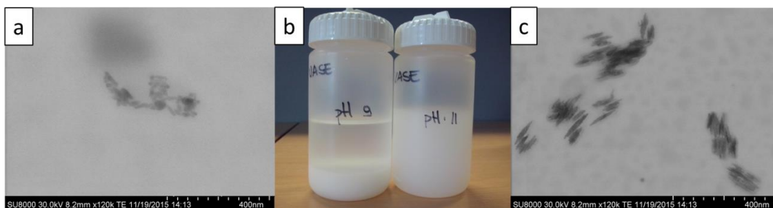
Fig. 3. FE-SEM images of SNC dispersion at (a) pH 9 and (c) pH 11 and sedimentation properties (b).
