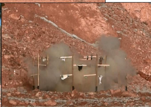
Figure 6.4. Pictures of the detonations of black powder, dynamite and ANFO explosives, extracted from the corresponding recorded videos. Each picture corresponds to the frame located approximately at 300 ms after initiating the detonation.
