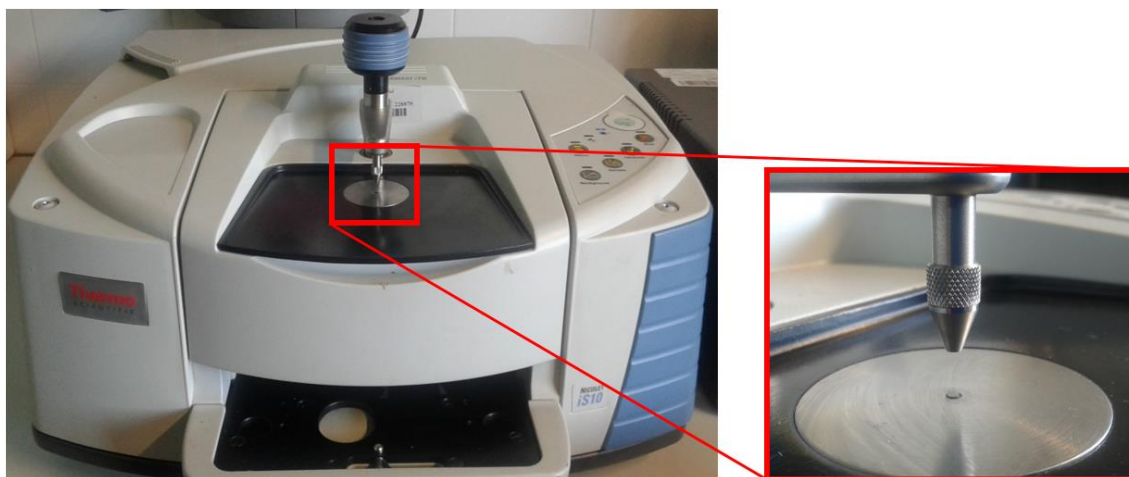
Figure 5.2. FTIR spectrometer equipped with ATR accessory (ATR zoomed).
