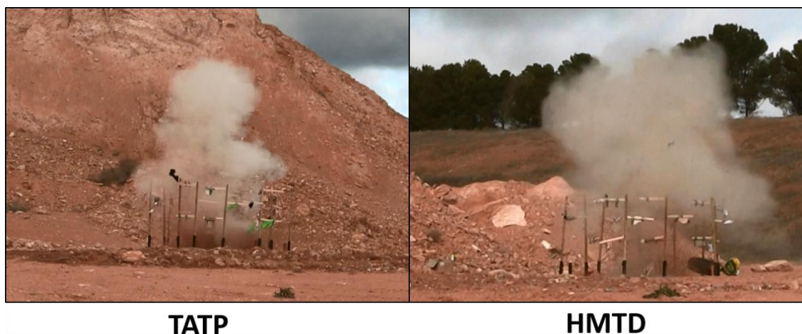
Figure 6.3. Pictures of the detonations of TATP and HMTD explosives, extracted from the corresponding recorded videos. Each picture corresponds to the frame located approximately at 300 ms after initiating the detonation.
