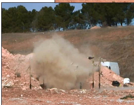
Figure 6.4. Pictures of the detonations of black powder, dynamite and ANFO explosives, extracted from the corresponding recorded videos. Each picture corresponds to the frame located approximately at 300 ms after initiating the detonation.
