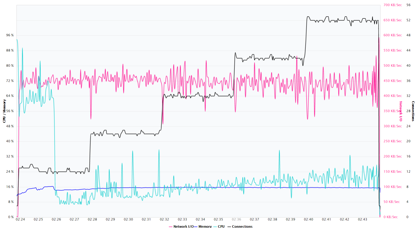
FIGURE 5. Engine Health Report for SPIDEPMS-T1-HB. The coloured lines represent various parameters: purple: bandwidth traffic; blue: memory load generated by users; light blue: CPU load generated by users; black: active connections within the test.
