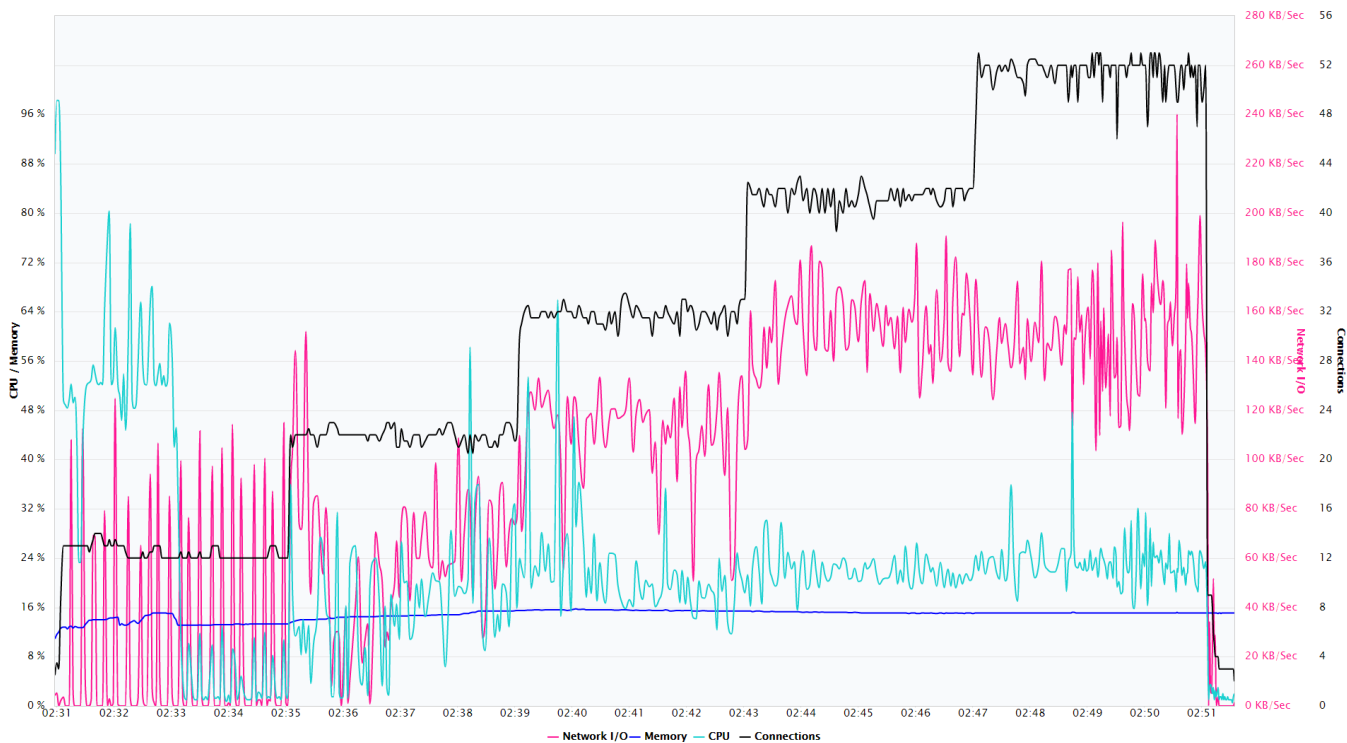
FIGURE 6. Engine Health Report for SPIDEPMS-T2-SQL. The coloured lines represent various parameters: purple: bandwidth traffic; blue: memory load generated by users; light blue: CPU load generated by users; black: active connections within the test.
