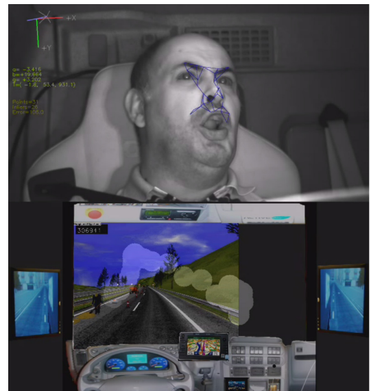
Fig. 6: Example of face pose estimation and gaze estimation, with fixation point on the scene.
