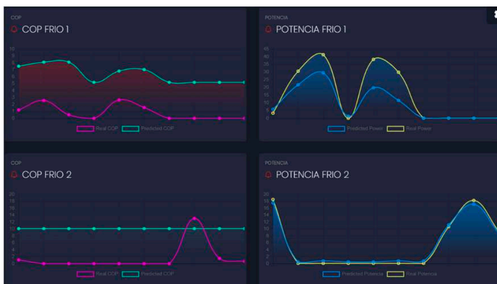
Figure 9. Time–domain evolution of variables ‘COP’ and ‘potency’ for coolers 1 and 2.
