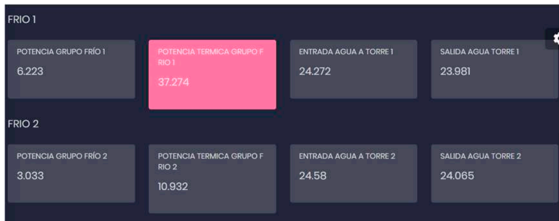
Figure 10. An example with an abnormal value highlighted.
