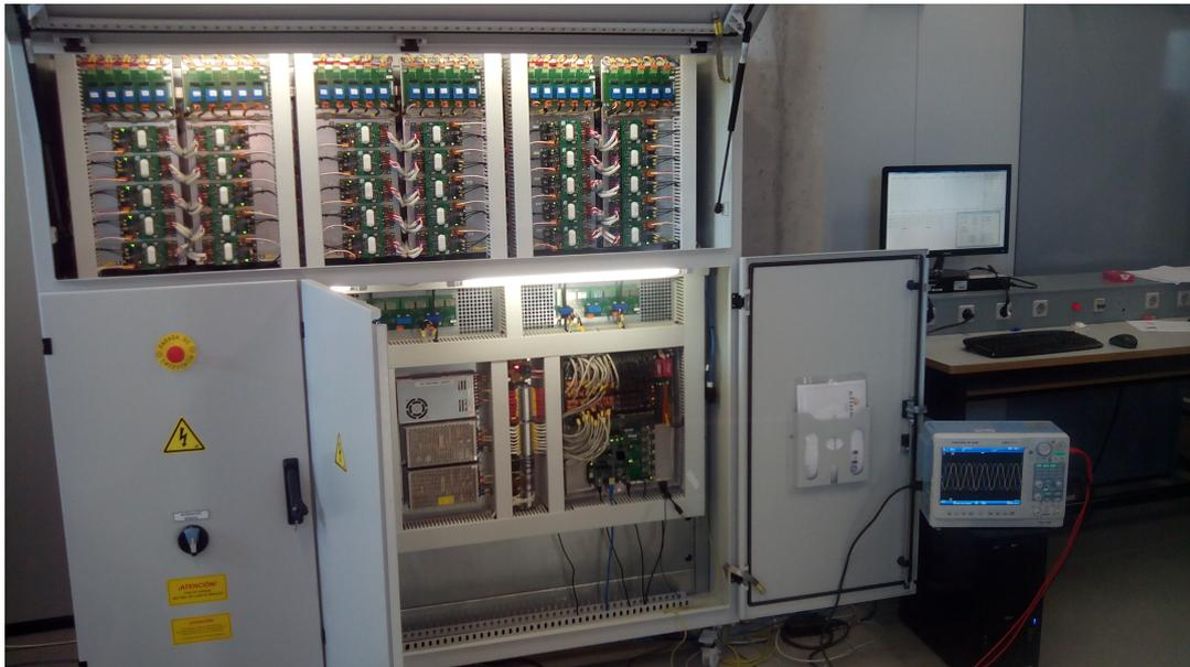
Figure 6.7: Modular Multilevel Converter prototype with five cells/arm.
