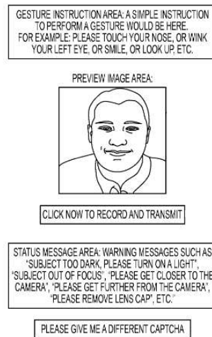
Figure 2.16: Webcam-CAPTCHA design (Greenblatt and Lagares-Greenblatt, 2012). The user is requested to perform some gestures in front of the camera.
