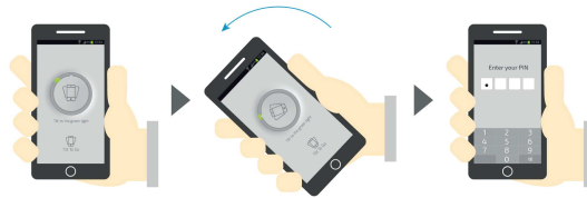
Figure 2.18: Physical CAPTCHA, or CAPPCHA design (Guerara et al., 2017). The user is asked to rotate her mobile device to a certain degree prior to access some other security measure.
