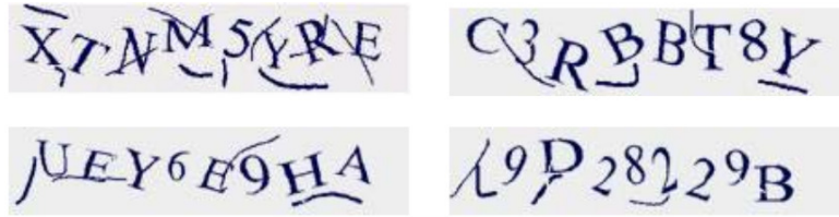
Figure 2.22: Example from the Microsoft CAPTCHA in 2008 (Yan and Ahmad, 2008). Note the lines drawn at random to try to prevent segmentation.
