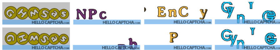
Figure 2.8: Some examples from HelloCAPTCHA, showing two frames for each. Some characters change position and orientation, and in some challenges, not all the characters are visible at the same time. This measures try to prevent a typical OCR attack over a single frame.
