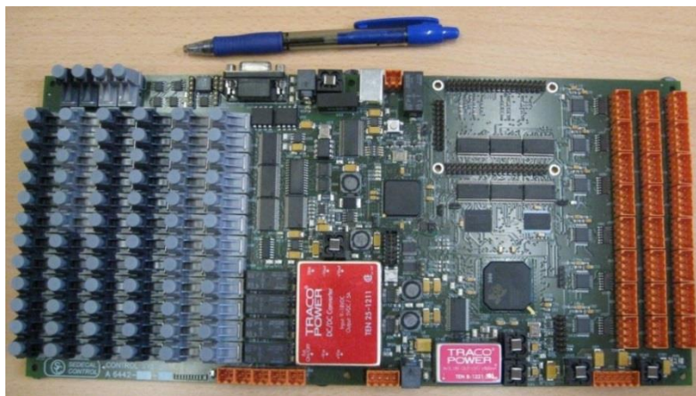
Figure 6.3. Control board for the DNPC converters, which is based in DSP+FPGA.
