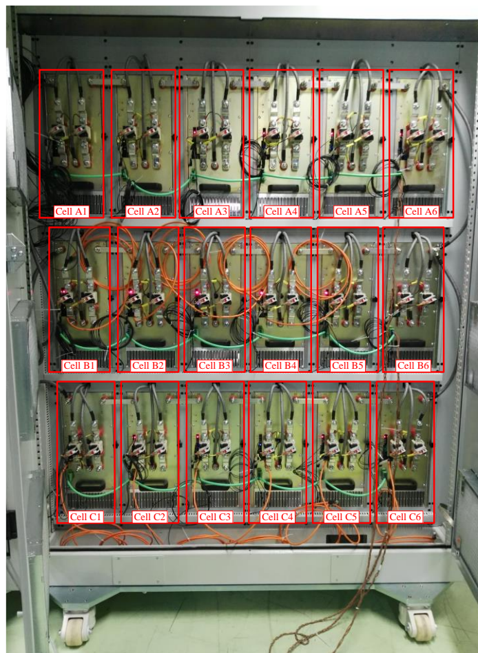
Figure 6.10. Illustration of the six-cells CHB converter developed by Sedecal Control.
