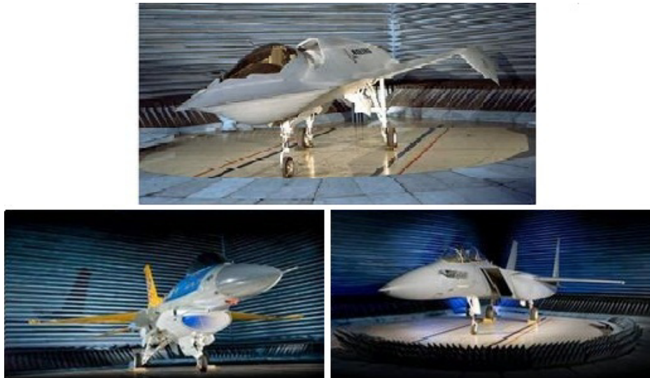
Figura 2.18: RCS Measurement Facility Boeing Phantom Works (obtenida de [99])
