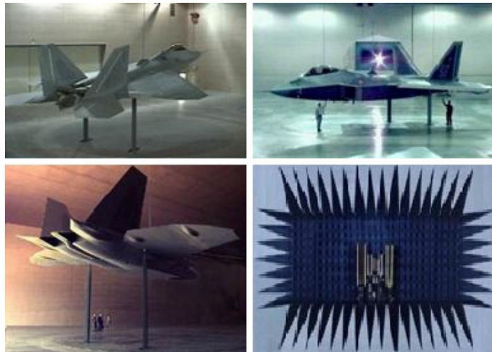
Figura 2.17: Aircraft RCS Functional Test Facility - Lockheed Martin Aeronautical Systems (obtenida de [98])
