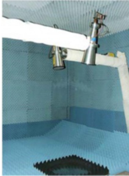
Figura 2.6: Bistatic Measurement Facility - DLR (obtenida de [34]).
