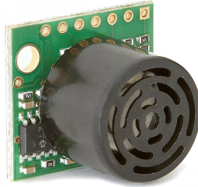
Figure 3.12: PROPINA: Sonar Range Sensor.
