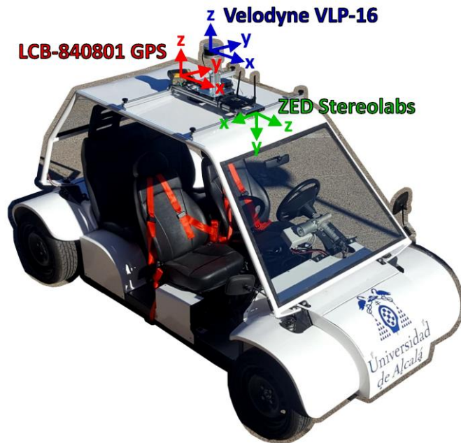
Figure 4.4-7 Frames Orientation and position of the main sensors in the vehicle
