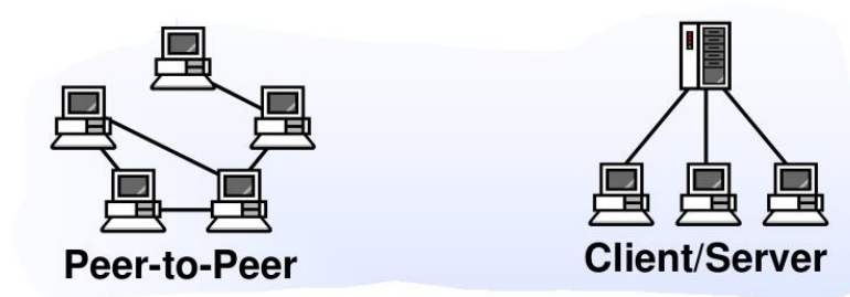
Figure 3.2-2 Peer-to-Peer vs Client/Server architecture
