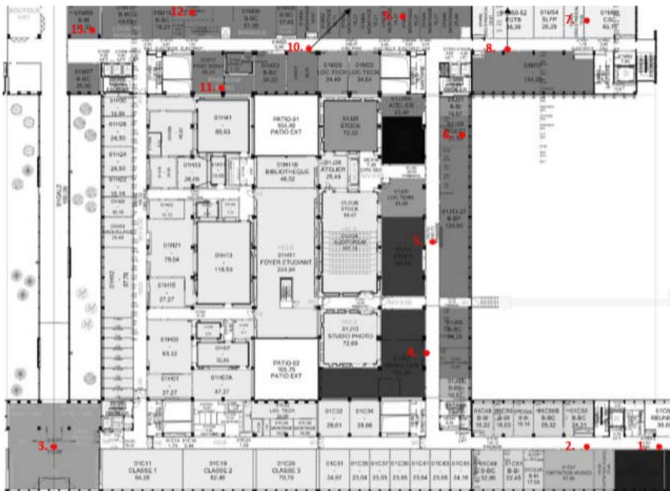
Figure 133 Placement Access Points for Floor 1 in Building PUVQ
