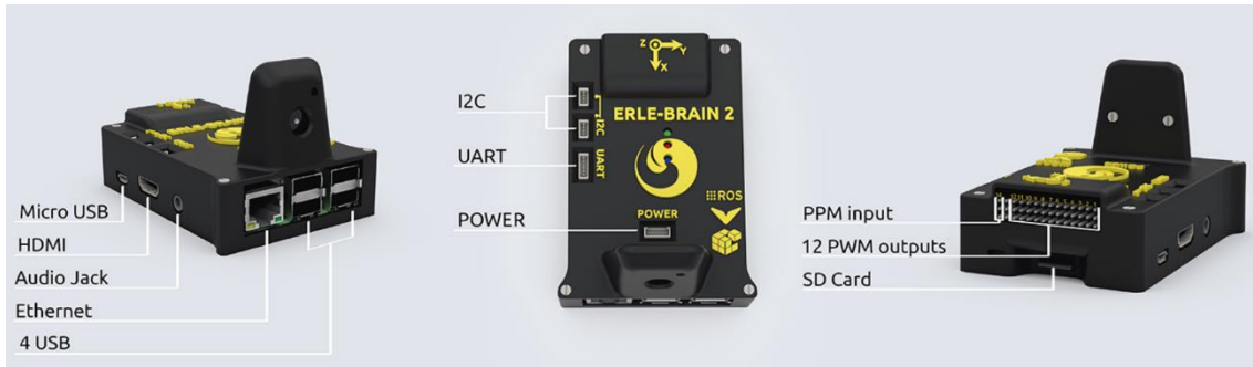
Figure 2. 10. Communication Units of the ErleBrain 2.
