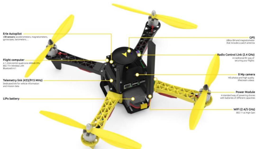
Figure 2. 6. Hardware parts of the ErleCopter.
