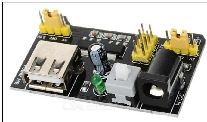
Figura 2.1-1: MB102 Breadboard.
