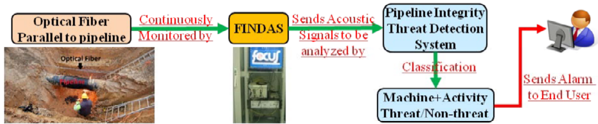
Figure 1. PIT-STOP surveillance system architecture.
