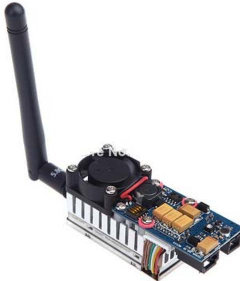
Figura 20: Transmisor 5.8GHz 2000mW
