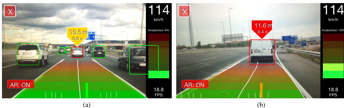
Figure 5.4: Examples of vehicle detection. (a) Driver keeps a relatively close distance (19.5 meters, 0.6 seconds) that is depicted in yellow colour. The module also detects 6 vehicles in the same frame, indicative of high traffic density. (b) Driver is at a very close distance to ahead vehicle, depicted in red colour. DriveSafe also emits an alerting sound on these dangerous cases.
