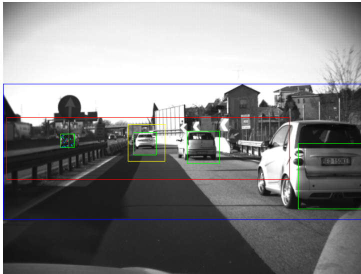
Figure 4.3: Example of the three vehicle detection stages working. Green boxes represent detections, blue the near-window, red the far-window, yellow the intermediate window (vehicle-specific) and the points depicted in blue in the vehicle of the left represent Optical Flow.
