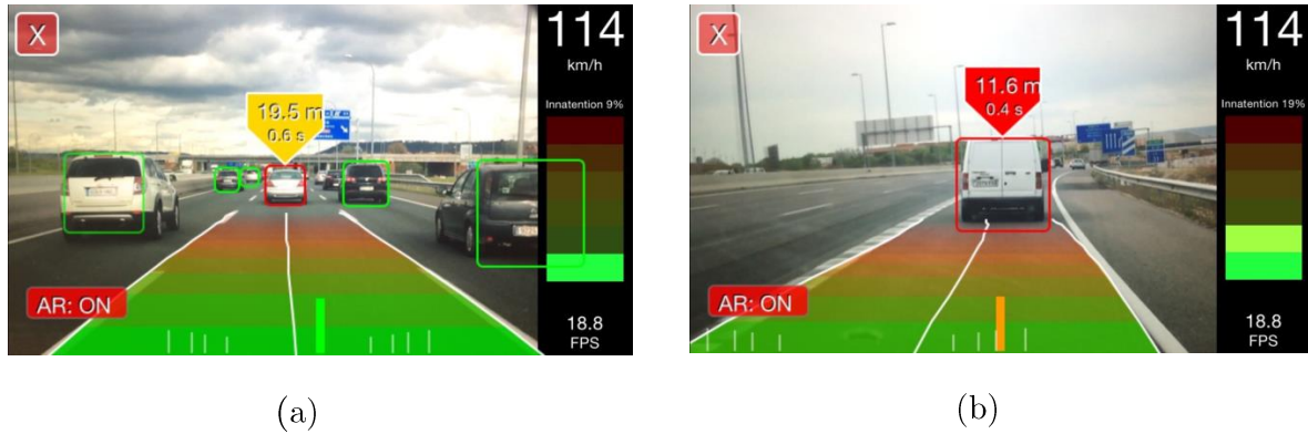
Figure 2. 9: Examples of vehicle detection. (a) Driver keeps a relatively close distance (19.5 meters, 0.6 seconds) that is depicted in yellow colour. The module also detects 6 vehicles in the same frame, indicative of high traffic density. (b) Driver is at a very close distance to ahead vehicle, depicted in red colour. DriveSafe also emits an alerting sound on these dangerous cases.
