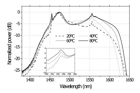
Figure 3. SC spectrum for different temperatures. The pump input power is always 2.1 W. Each curve has been normalized by its own maximum to show more clearly the increase of the SC width. The inset shows how pump depletion is less intense as the temperature grows.
