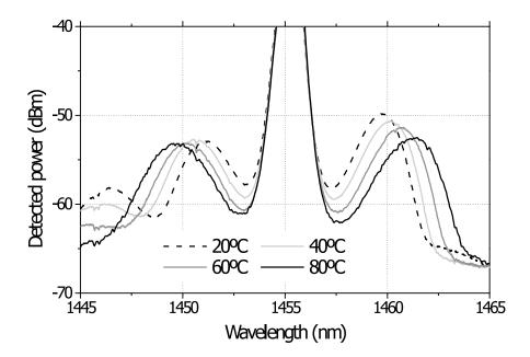
Figure 2. MI spectrum around the pump wavelength for different temperatures. As the temperature grows, the asymmetry between the MI side lobes is less evident.
