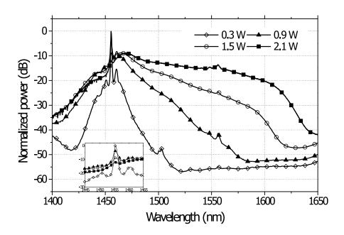
Figure 1. SC spectrum with different pump powers at room temperature ( $\simeq 20$ C). All the curves have been normalized to the same peak value. Inset shows how increasing pump power leads to a more efficient pump depletion.
