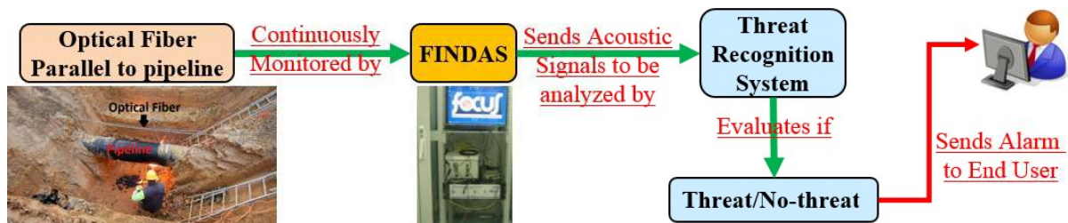
Figure 1. PIT-STOP surveillance system architecture.
