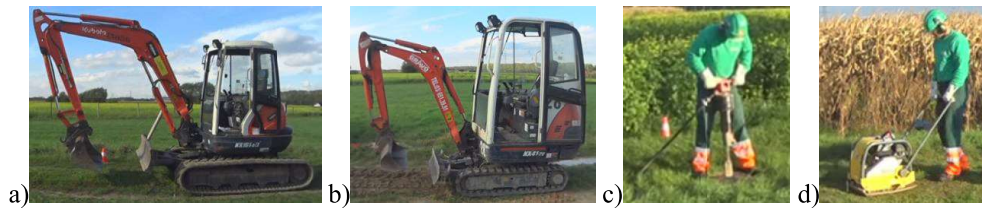
Figure 2. Machines used for the fields tests: a) Kubota KX161-3 (~5000kg; 5.54x2.53x1.96m length/height/width), b) Kubota KX41-3V (~1500kg; 3.66x2.28x0.99m length/height/width), c) Pneumatic hammer, d) Plate compactor
