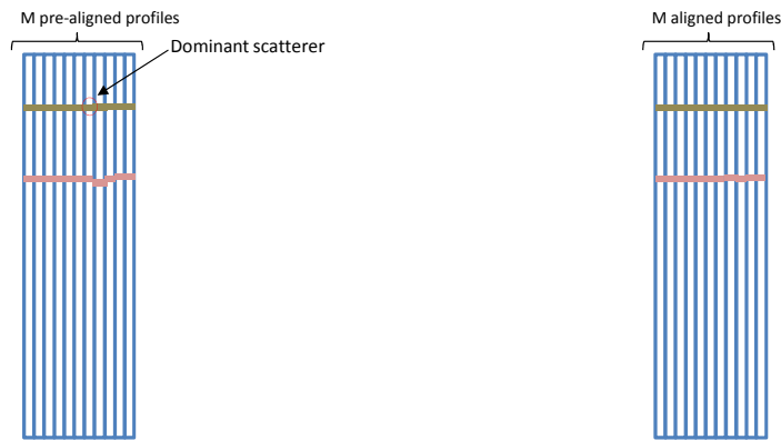
(d) Select a dominant scatterer and proceed with a fine alignment with respect to it. (e) The M profiles of the HRRP measurement are finally aligned.
