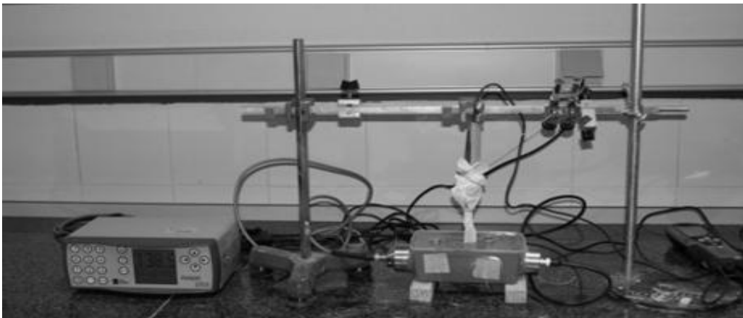
Figure 1: Ultrasonic and temperature monitoring setup.
