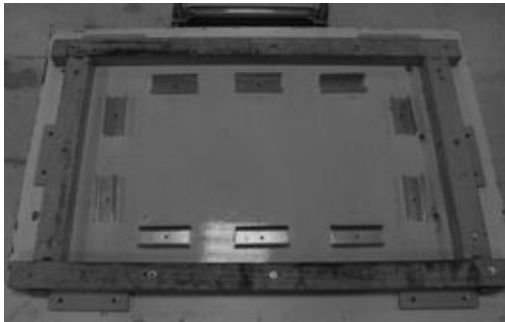
Figure 3a: Kraai Slab Test
