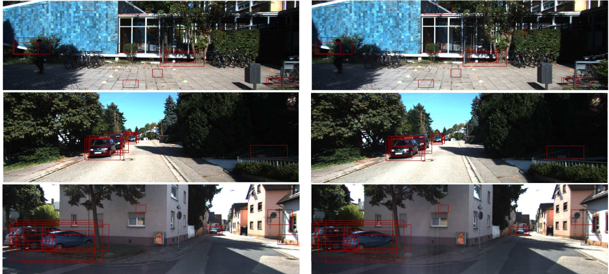
Figure 5.20: Examples of matched candidates on the left and right disparity images when employing our stereo consistency check. The bounding boxes are detections of cars when using the features C8B1 . As it can be seen, there are true and false positives found in the married-matching. Consequently, there are slight increases in precision because several high-scoring false positives are detected on both views of the stereo and cannot be filtered out with our approach.
