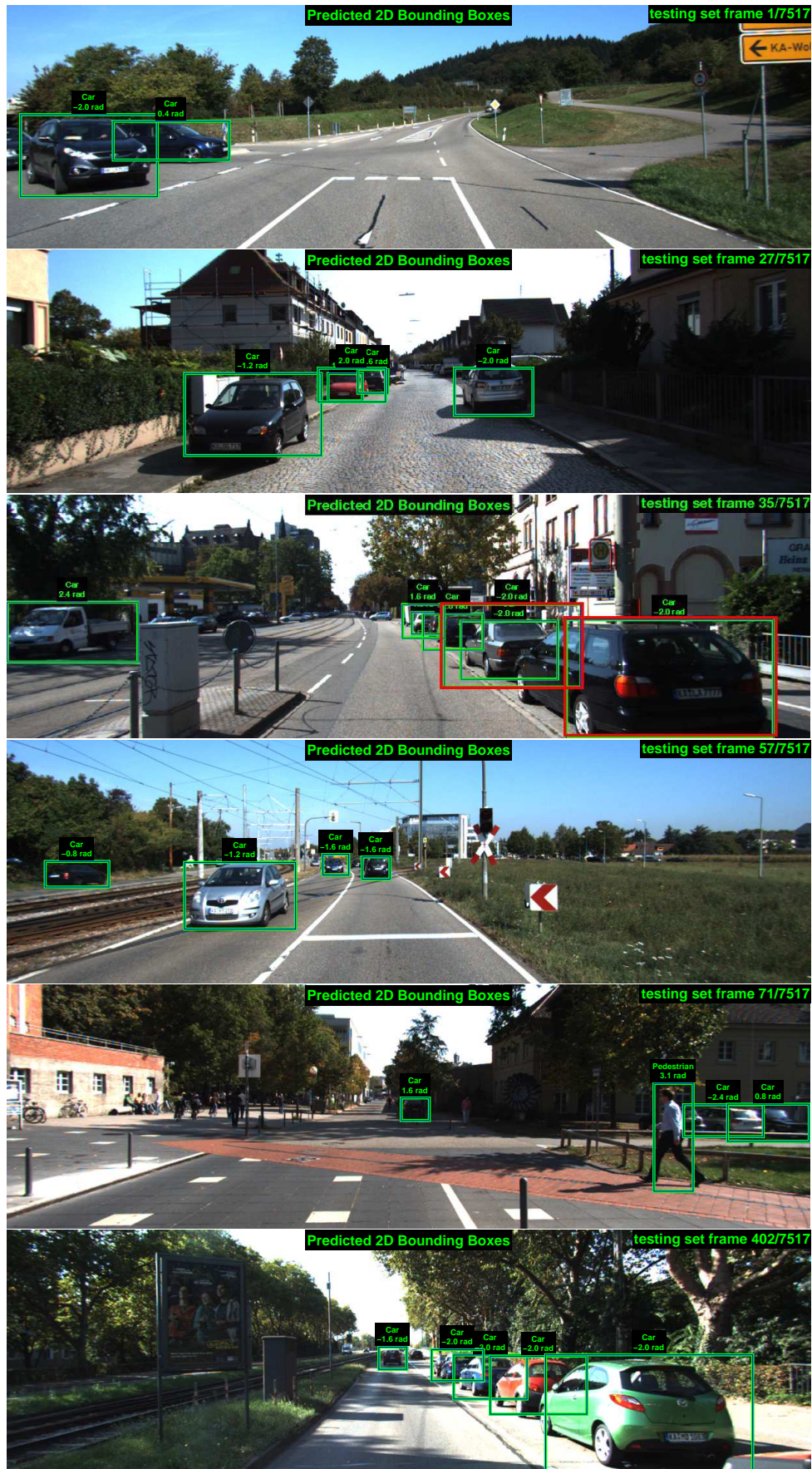
Figure 5.10: Examples of predicted labels in KITTI testing frames with TPs, FPs and FNs.
