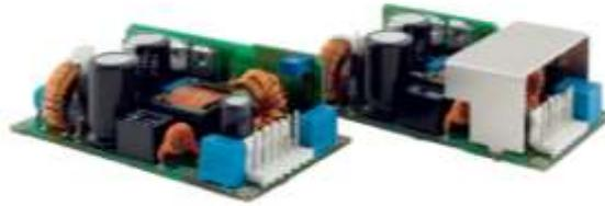
Figura 136: Conversor 230Vac a 24Vdc
