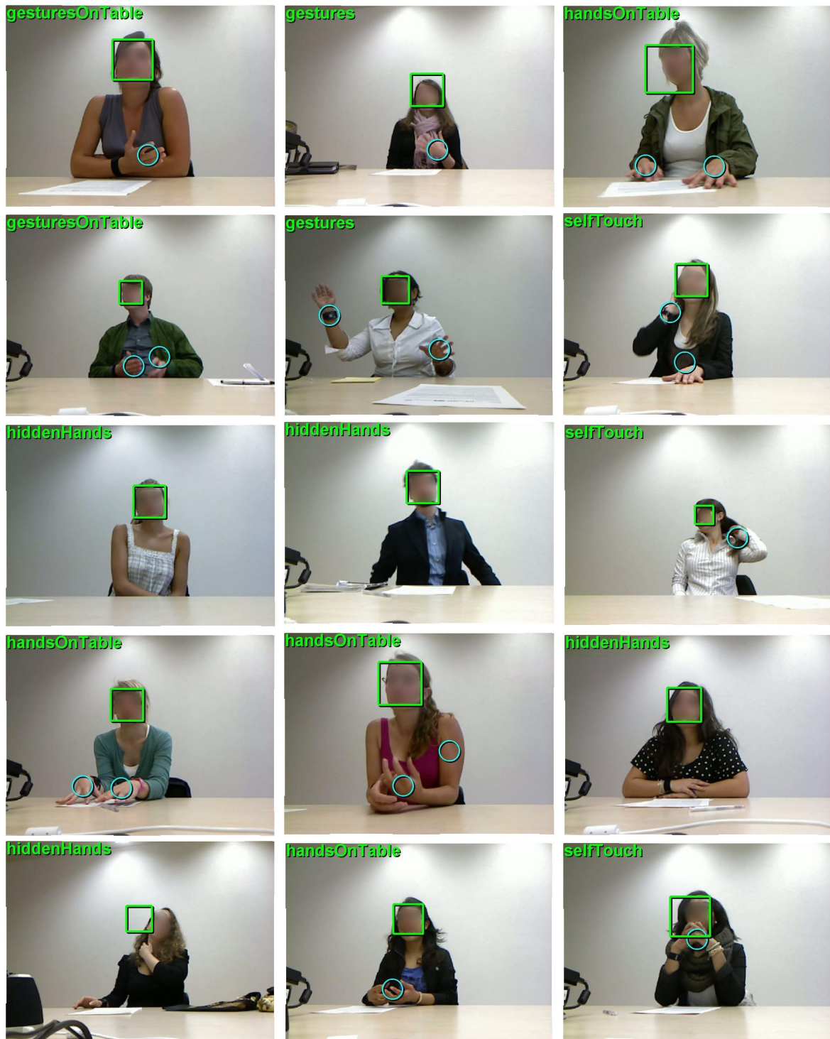
Figure 6.27: Frame results in the RGBD case. Overlaid to RGB images are the hand and face position, and the detected ongoing activity. The last five RGB images row shows failure examples (first: positive from the hand detector, second: missed hand detection; third: incorrect face detection; fourth and fifth: merged hands). Best viewed in color.
