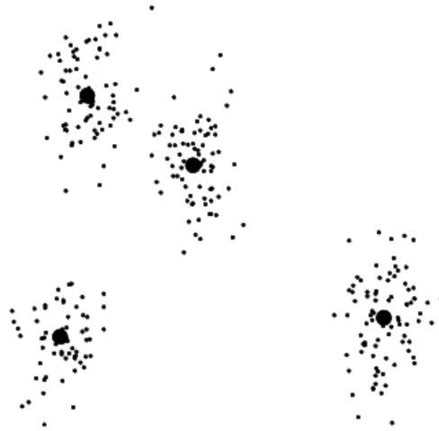
Figure 2.1: Extended K-means 2D example. With an unspecified number of input classes, but with a distance threshold parameter, the number of groups is estimated. Modified figure taken from [Pelleg and Moore, 2000].
