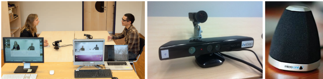
Figure 4.2: Setting and data collection. Audio and video for interviewer and participant were recorded and synchronized. Left: general setup. Center: kinect and HD cameras. Right: microcone.
