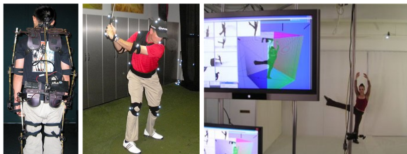
Figure 3.2: Motion capture techniques. Left: physical. Center: optical. Right: markerless
