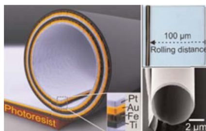
Figure III.4. Schematic diagram of a rolled-up microtube consisting of Pt/Au/Fe/Ti multilayers on a photoresist sacrificial layer ( left ). Optical microscopy and SEM images of a rolled-up Pt/Au/Fe/Ti microtube ( right ). Reprinted with permission from reference 24
