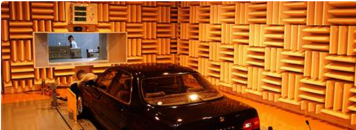
FIGURE 4, ACOUSTIC TEST CHAMBER
