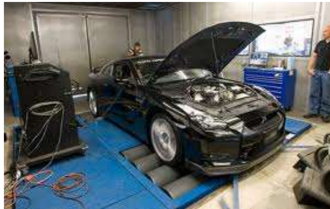
FIGURE 5, EXHAUST EMISSIONS MEASUREMENT ON A CHASSIS DYNAMOMETER
