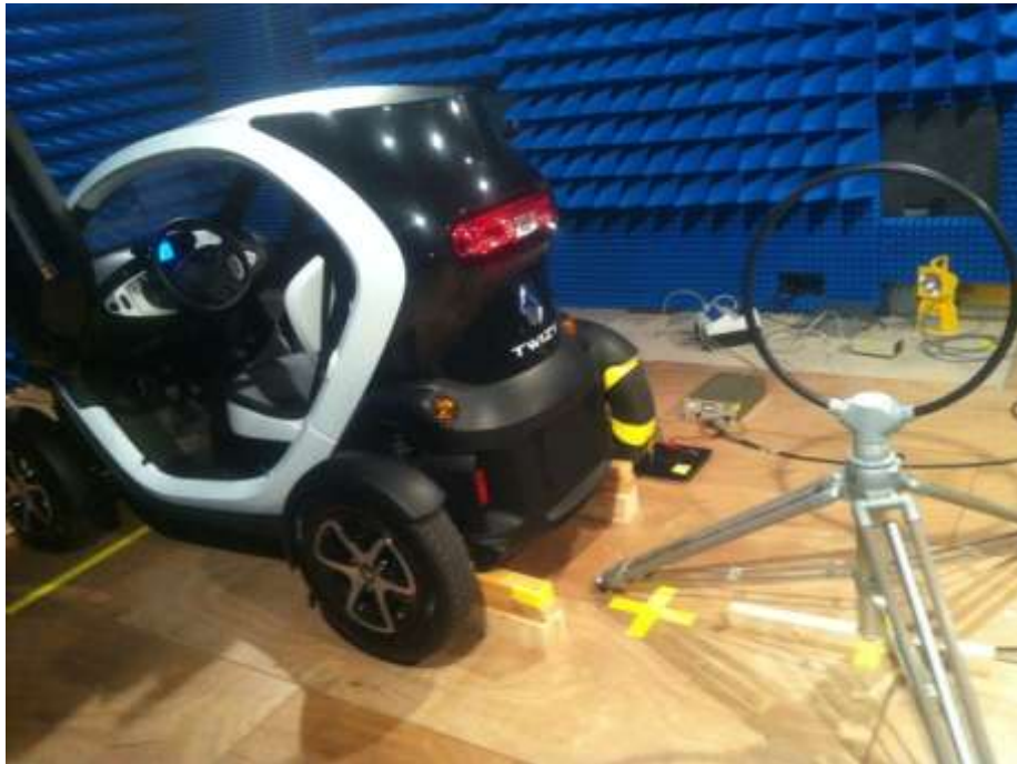
FIGURE 16, ROHDE &amp; SCHWARZ LOOP ANTENNA DURING EXPERIMENTS WITH A RENAULT TWIZY
