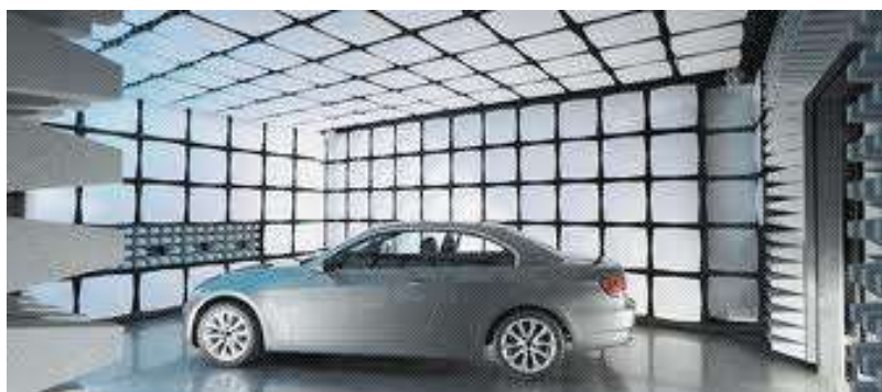
FIGURE 6, EMC SEMI-ANECHOIC TEST CHAMBER
