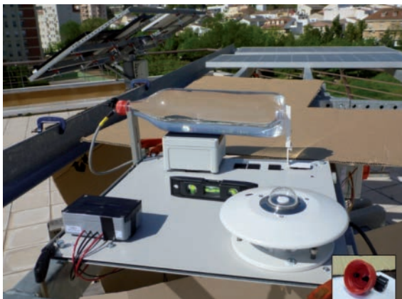
Figure 36. Set-up of experiment with bottle filled with tap water and the SolWat sensor underneath to measure irradiance in the bottom of the bottle and water temperature (17 th April 2013)
