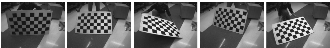
Figure 3.7: Samples of the set of images used to calibrate the camera with the Matlab Calibration Toolbox.
