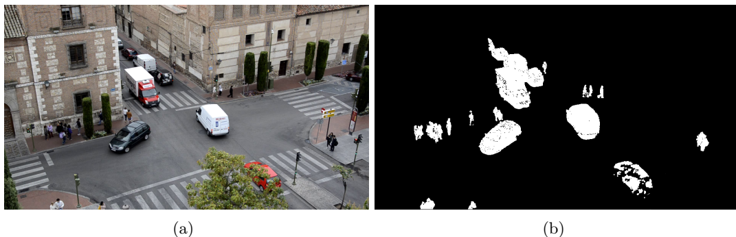
Figure 2.11: Example of blob merge due to partial occlusions and blob split due to a tree, after applying background subtraction. (a) Original image. (b) Foreground mask.
