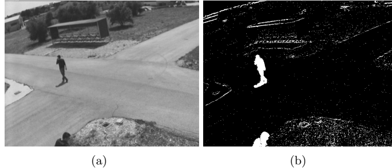
Figure 1.4: Background subtraction problems due to instabilities of the camera.
