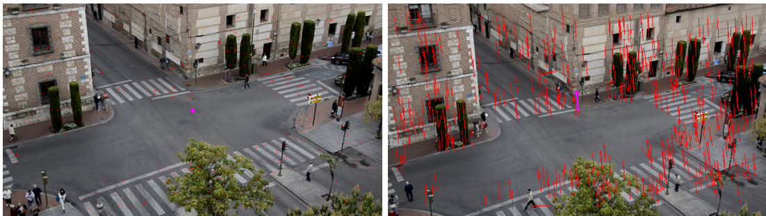
Figure 4.5: Example of detected pitch change. (a) Source image before the pitch variation. (b) Image after pitch variation and motion vectors.
