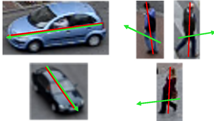
Figure 3.18: Angles used to differentiate between vehicles and pedestrian. Green arrowhead stands for velocity direction; Red line stands for main axis direction.
