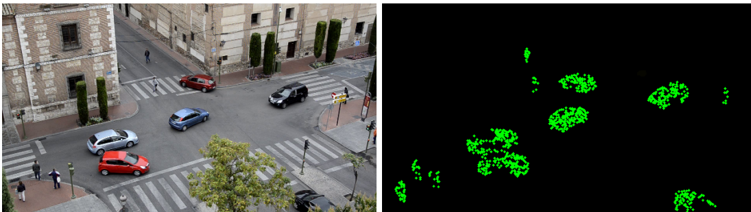
Figure 4.10: FAST features extracted from an image. (a) Source image. (b) Extracted features.
