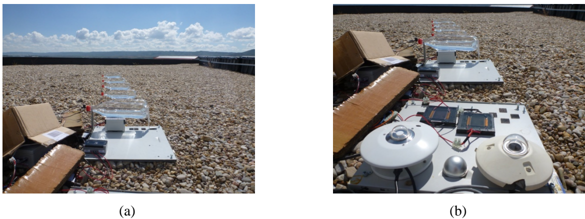
Fig. 39: Set-up of experiment with PET bottles filled with water with E.coli and the SolWat sensor unit 2 underneath one of them to measure irradiance in the bottom of the bottle and water temperature, along with the SolWat sensor unit 1 measuring sunshine duration, global irradiance and UV irradiance; and a weather station (21 st May 2013).
