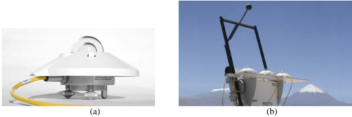
Fig. 9: a) Pyranometer; b) Sun tracker including a pyrliometer measuring direct radiation, two pyranometers measuring global, and a third pyranometer with the shading ball measuring diffuse radiation [33].
