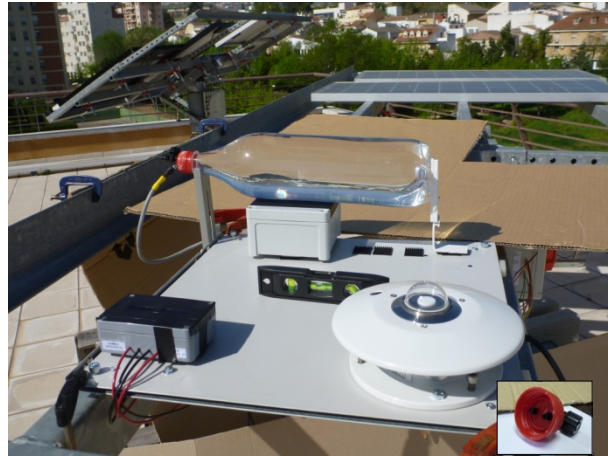
Fig. 36: Set-up of experiment with bottle filled with tap water and the SolWat sensor underneath to measure irradiance in the bottom of the bottle and water temperature (17 th April 2013).
