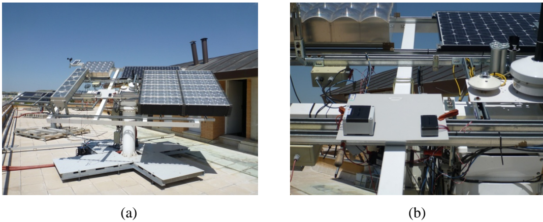
Fig. 31: Sensor units under calibration on the tracker at the outdoor solar facilities at University of Jaén, measuring I_{SC,Cell_1} , I_{SC,Cell_2} , I_{SC,Cell_3} , V_{OC,Cell_4} and T_{Cell_4} under natural sunlight (irradiance measured by the pyranometer in the tracker).
