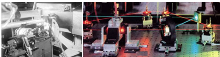
Figure 1.2 Left: the original flash photolysis apparatus ( Thrush 2003 ). Right: femtosecond spectroscopy setup in the Laboratory of Molecular Sciences at California Institute of Technology (see http://www.lms.caltech.edu ).
