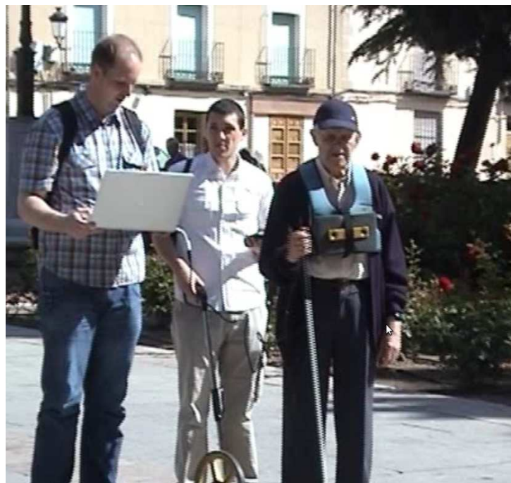
Figure 6.11: The stereo camera system is attached to chest of the visually impaired user by means of a non-invasive orthopedic vest. Then the camera is connected to a small laptop by means of a fireware cable.
