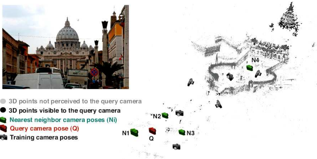
Figure 4.2: Given a large city-scale 3D reconstruction, we predict the visible 3D points for a query camera view by fusing both geometric and appearance information from multiple neighbor cameras. Best viewed in color.
