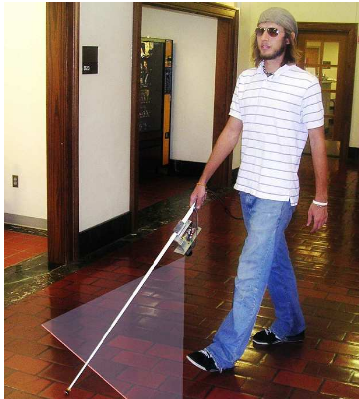
Figure 6.2: A portable indoor localization aid for the visually impaired based on the fusion of several sensory modalities (gyroscopes, pedometer and a laser scanner).
