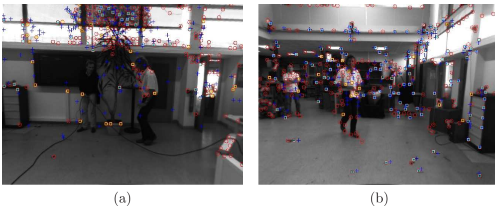
Figure 5.16: (a) In this area localization is more difficult, mainly due to the lack of textured features. (b) Even though there are some persons walking in the environment occluding some visible 3D points, the algorithm is able to find correct pose estimates without problems. The red circles are the detected 2D features, the blue crosses represent the reprojection of predicted visible 3D points. The set of inliers putatives after solving the PnP problem are represented by cyan rectangles, whereas the outliers are represented as yellow rectangles. Best viewed in color.
