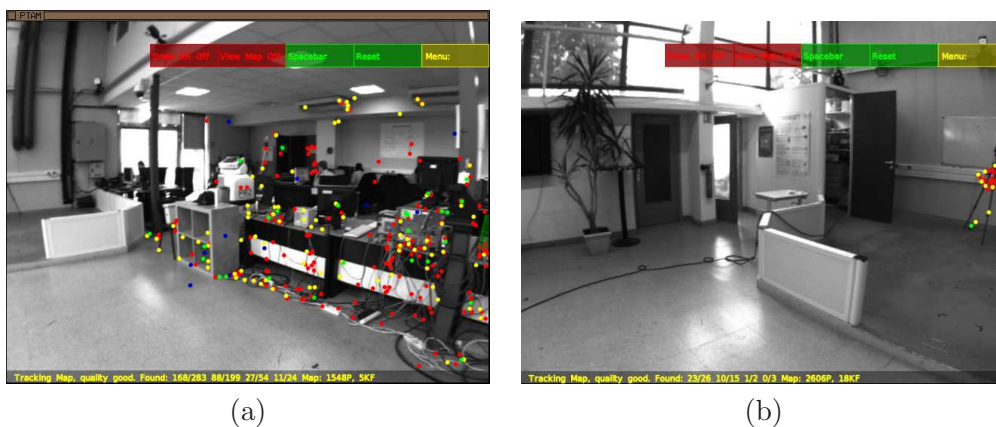
Figure 5.21: PTAM Tracking Results: (a) One frame of the circular sequence where PTAM tracking was successful (b) One frame where PTAM tracking had severe problems and new 3D map points can not be added to the map.
