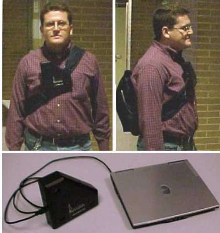
Figure 6.3: Wearable stereo device for 6-DoF SLAM for the visually impaired.
