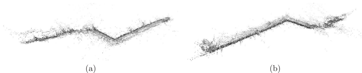
Figure 6.24: Different image views of the sparse 3D point cloud reconstruction from the Alcalá de Henares city-center dataset. Each 3D point is depicted by their grey image value when the point was added to the map for first time.
