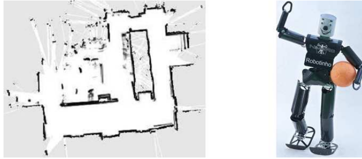
Figure 5.1: A learned grid map using noisy and short-range laser data acquired with the humanoid Robotinho .
