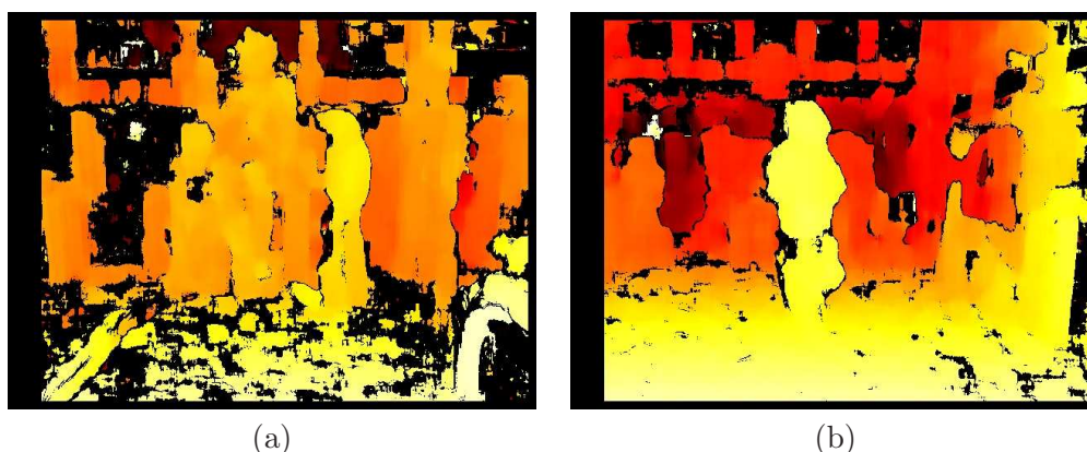
Figure 5.17: Disparity maps of two frames. Disparity is coded by using a hot color space representation. In this representation, close 3D points to the camera are depicted in yellow, whereas far points are depicted in red. Best viewed in color.
