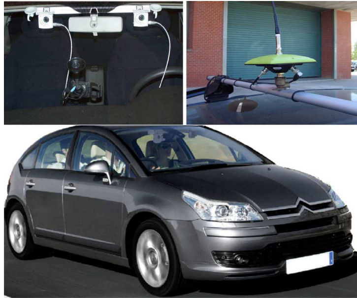
Figure 2.1: System architecture mounted on a commercial car. (Top left) Stereo vision system and low-cost GPS. (Top right) Ground truth RTK-GPS used for system validation.
