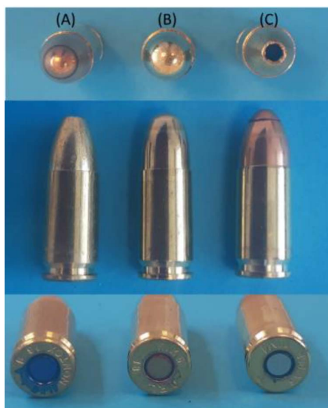
Figure 1 Images of the ammunition used (A) Sellier & Bellot, (B) Fiocchi, and (C) SeCa cartridges.
