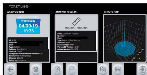
Figure 5 Image of the software interface with a display of the results of the shooting distance determination and the density map.
