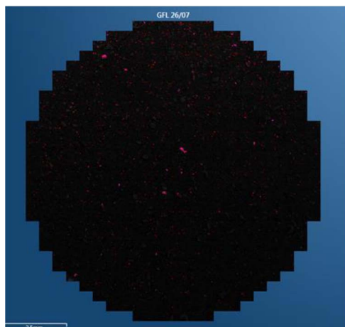
Figure 6 Distribution of copper (red spots) over a sample surface.
